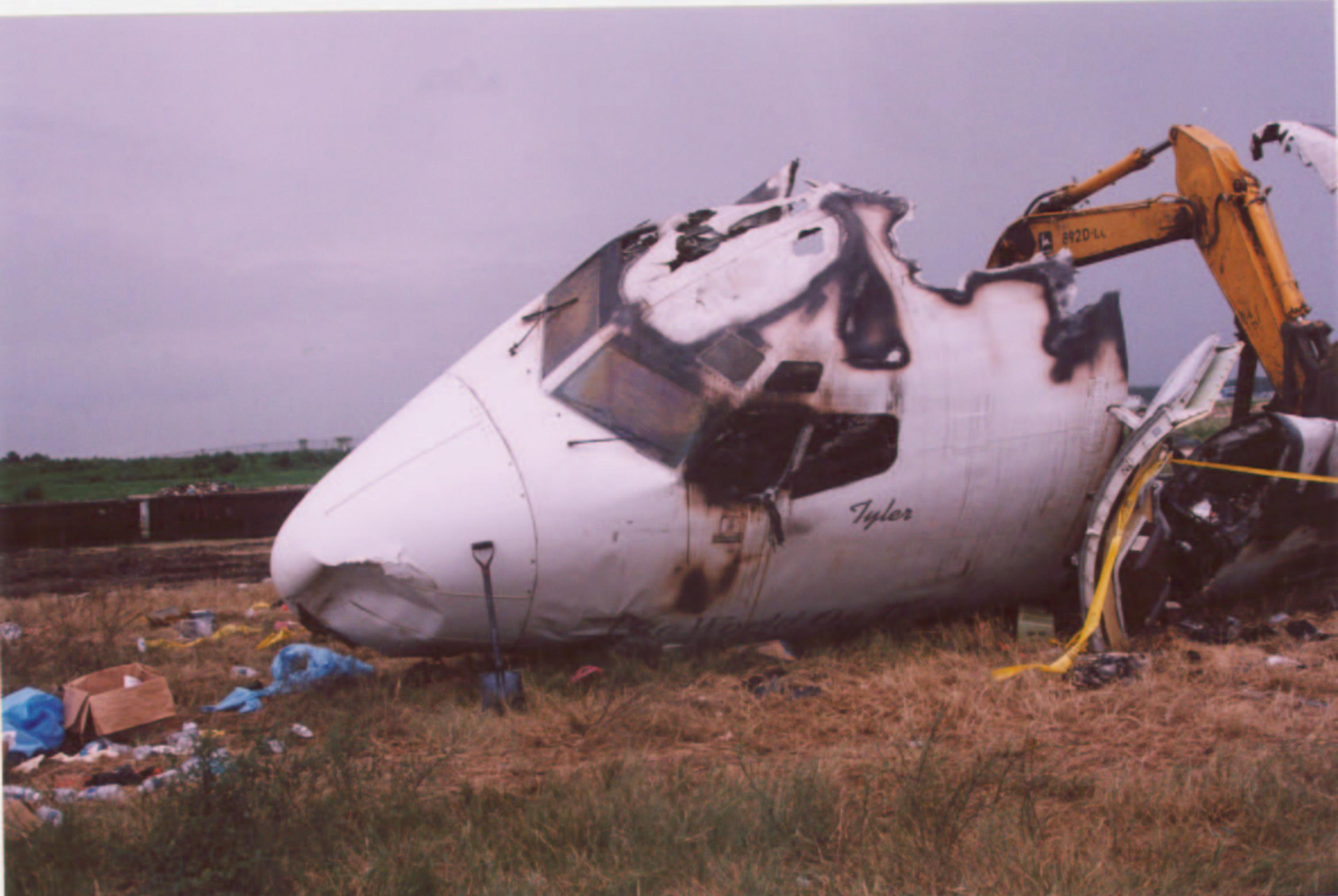
Appendix "B" Photo 9 - Close up of Left Fuselage Showing Damage to Radome
