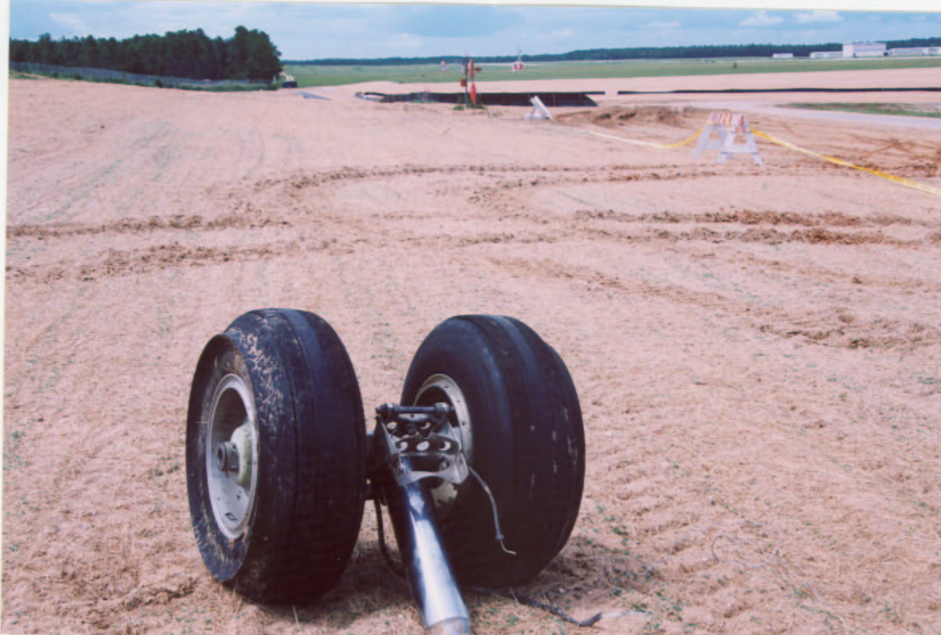
Appendix "B" Photo 18 - Nose Landing Gear Found on the Wreckage Path
