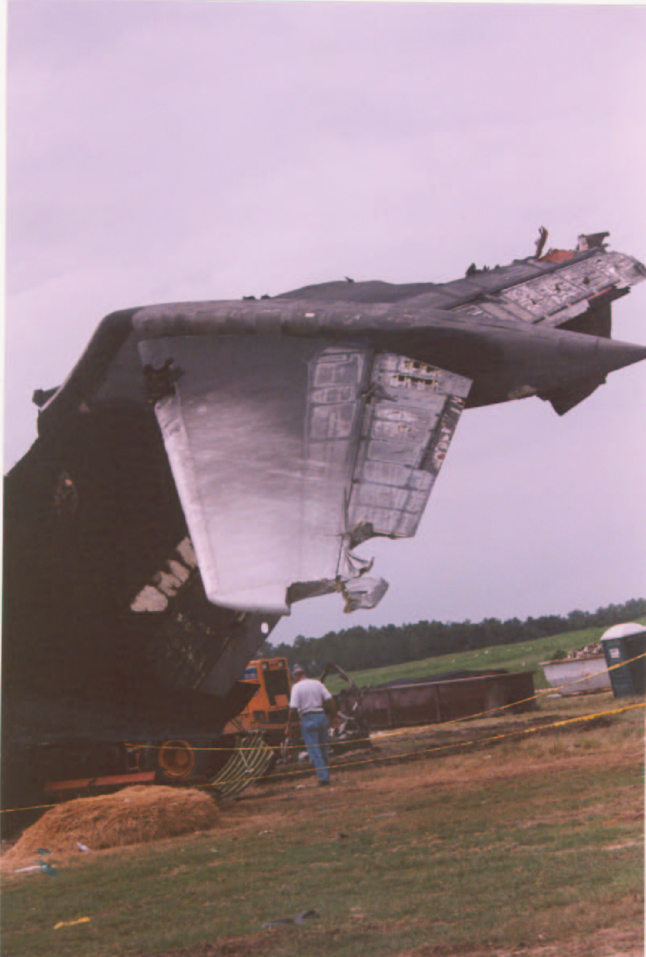
Appendix "B" Photo 15 - Damage to Left and Right Horizontal Stabilizer
