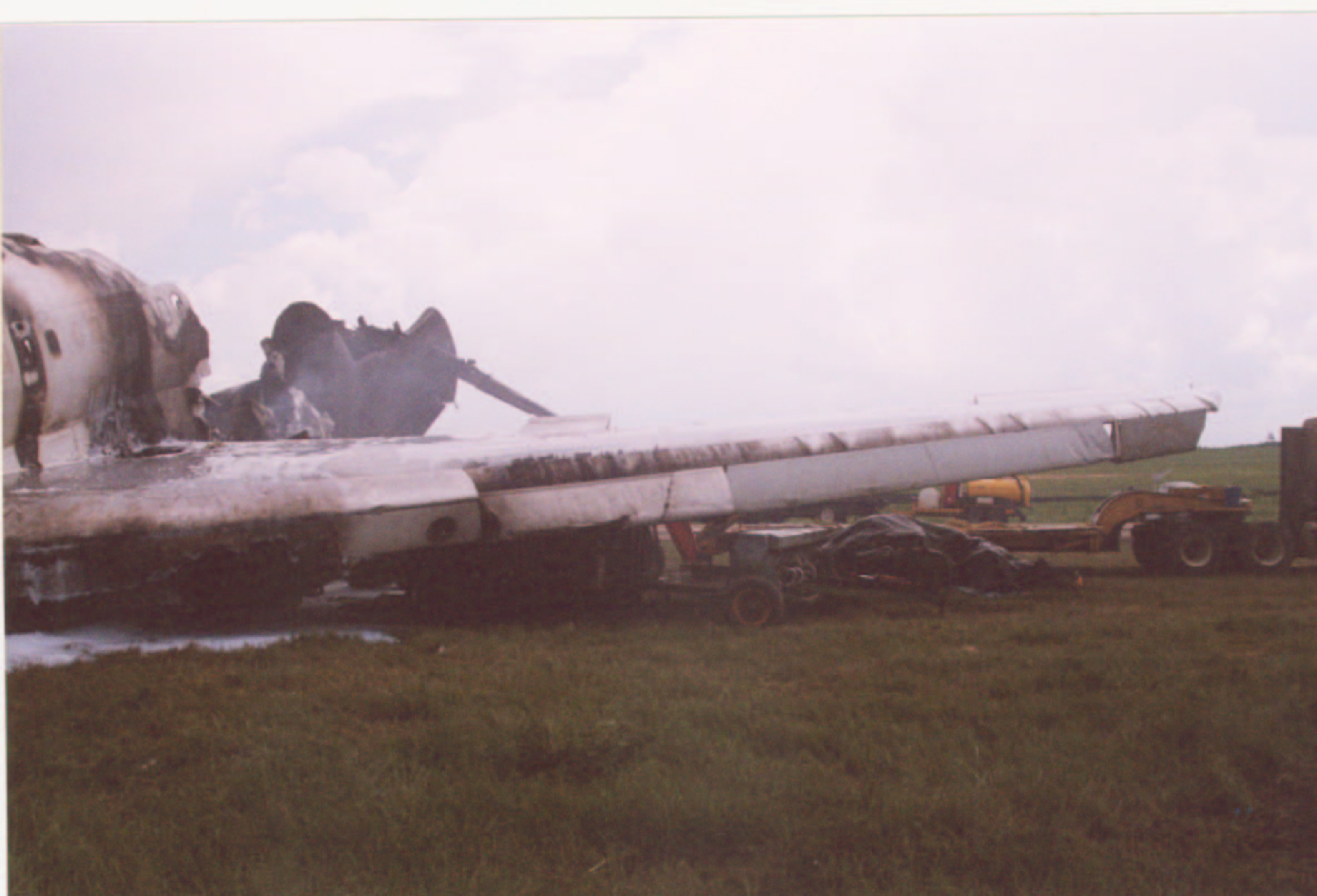
Appendix "B" Photo 12 - View Showing Damage to Left Wing Leading Edge
