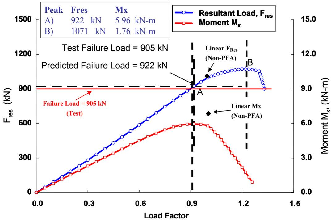
Figure A.1. Load and Moment vs. Load Factor for Full Scale Test Load Case
