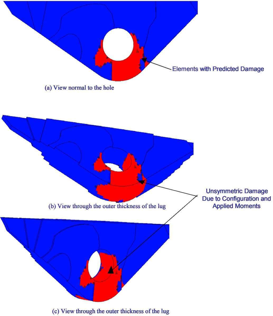
Figure A.2. Damage Prediction for Full Scale Test case from PFA
