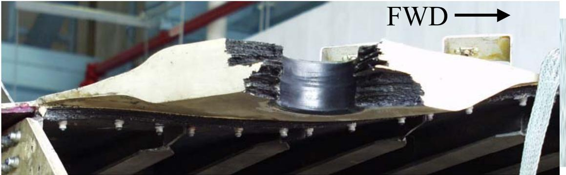
Figure A.3. AA 587 Right Rear Lug – Observed Failure
