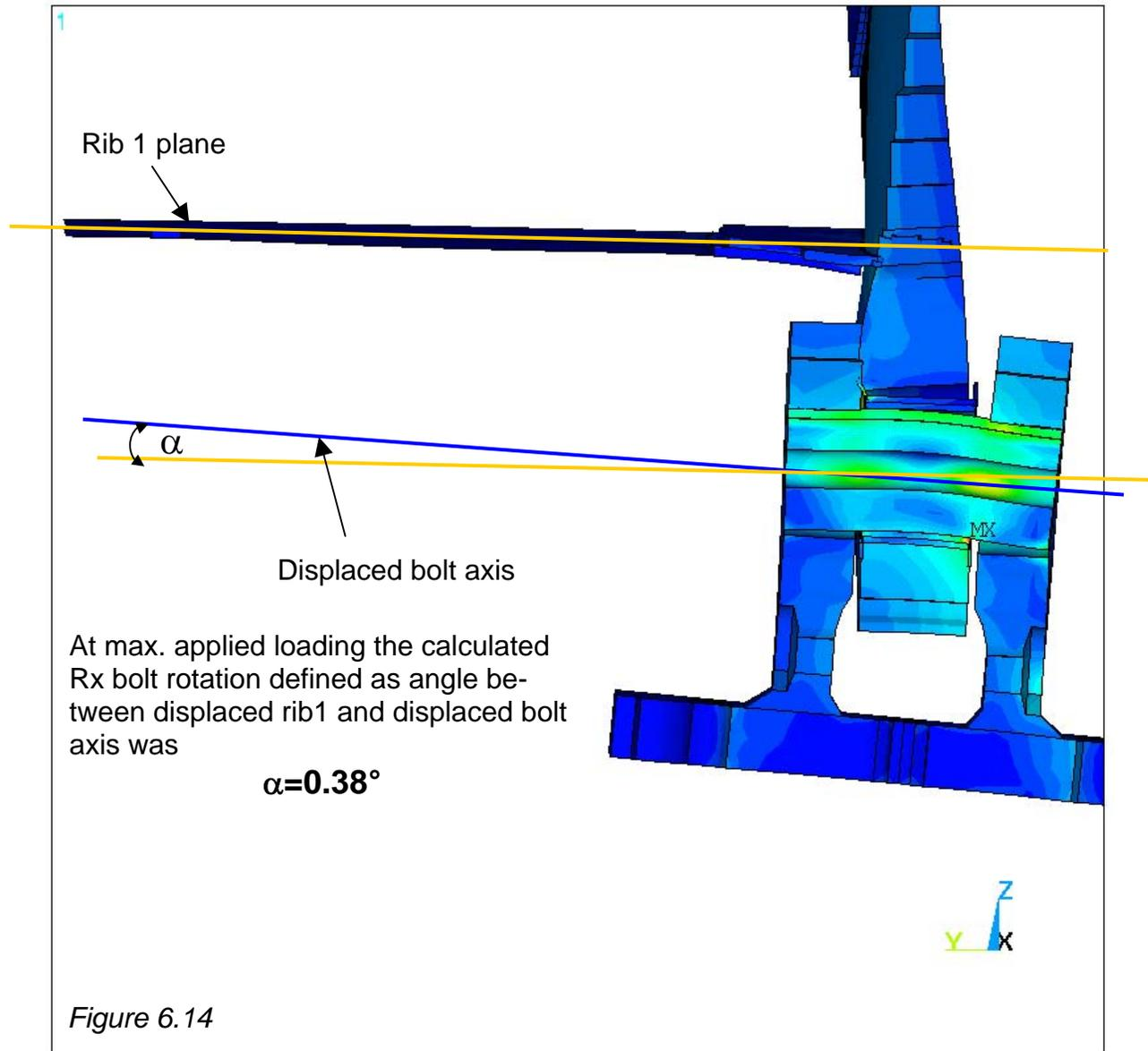
**Deformations are scaled up for a better understanding of the structure behaviour**
