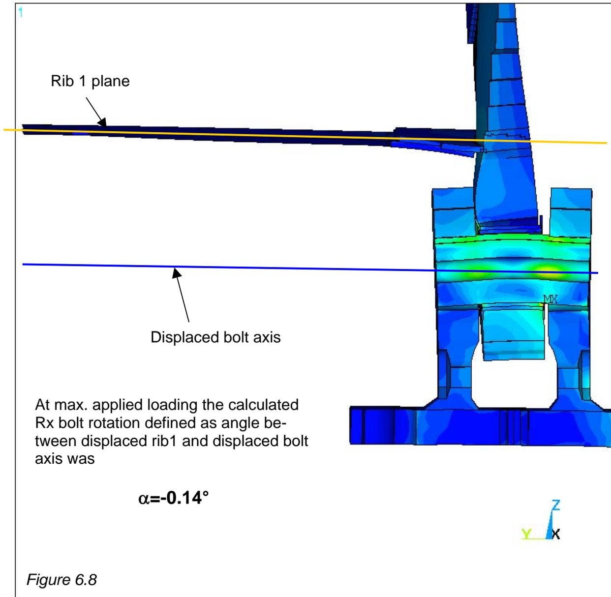
**Deformations are scaled up for a better understanding of the structure behaviour!**
