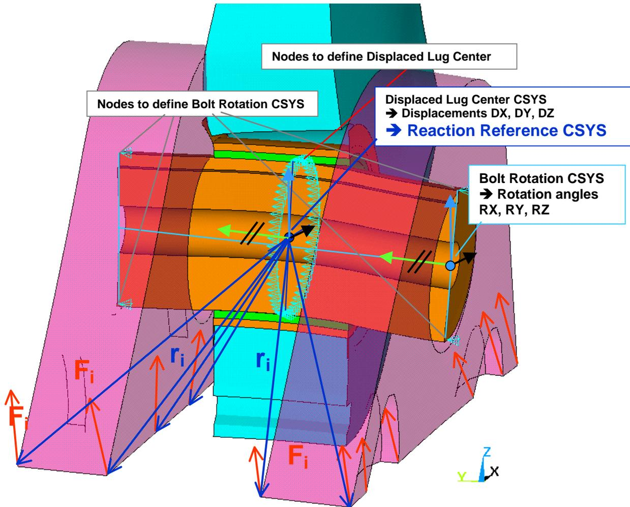
**Deformed structure! (Displacements scaled by a factor 10)**
