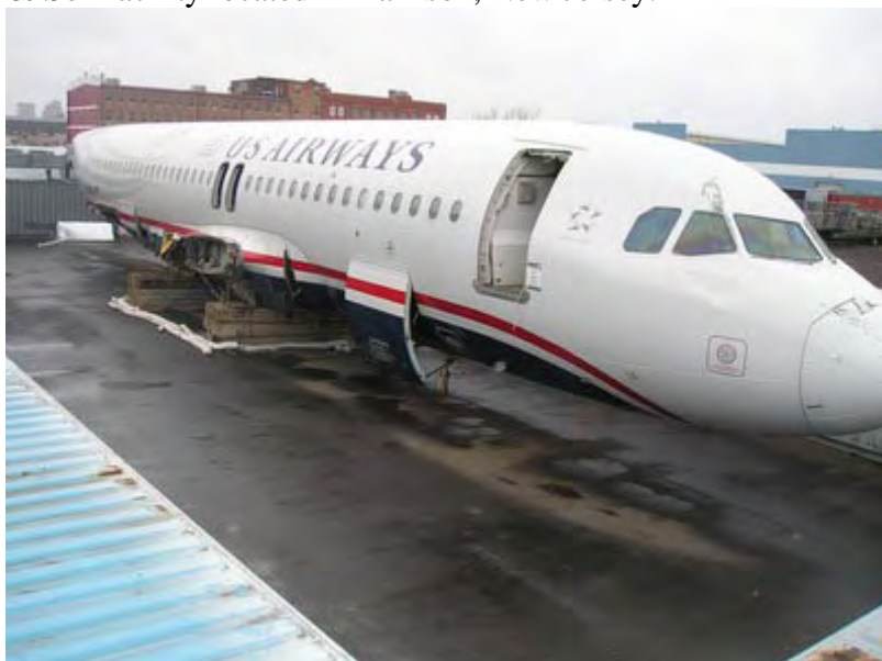
Figure 3 – US Airways N106US After removal of the wing and stabilizers.
