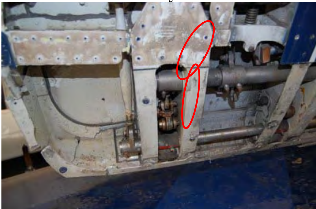
Fractured fork fitting at frame 55A
