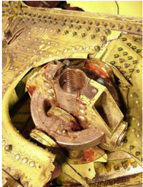
Figure 2. Acme Nut Installed in Accident Aircraft
