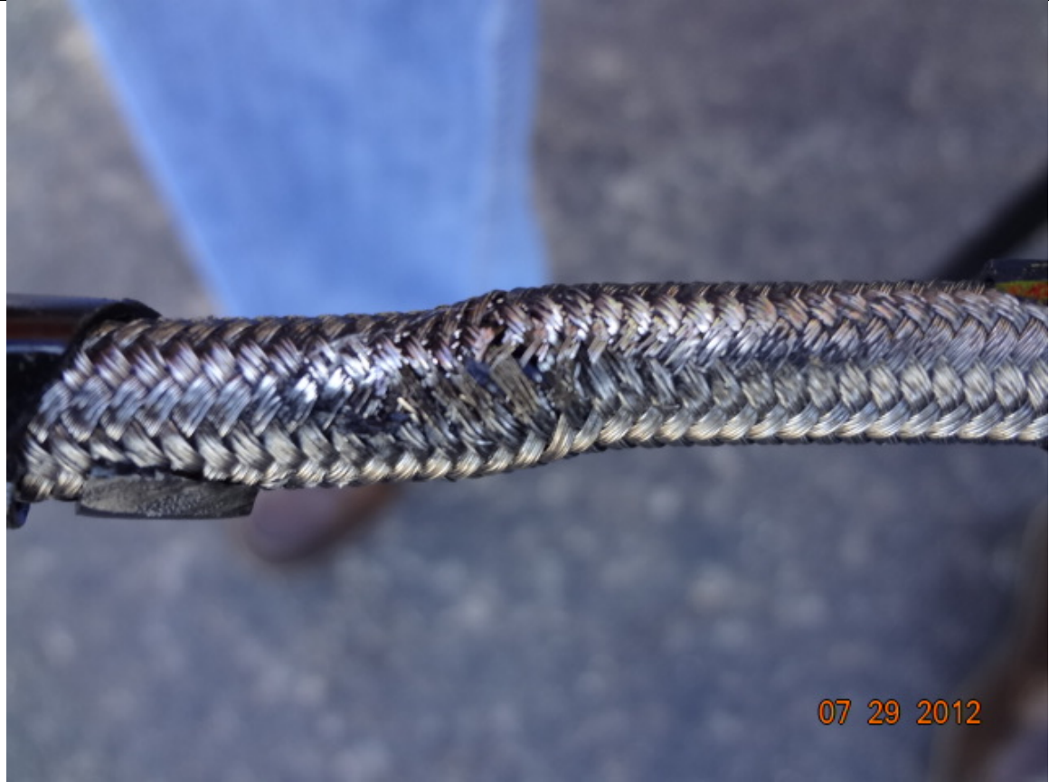
Photo 11: N379SW ruptured hydraulic line
