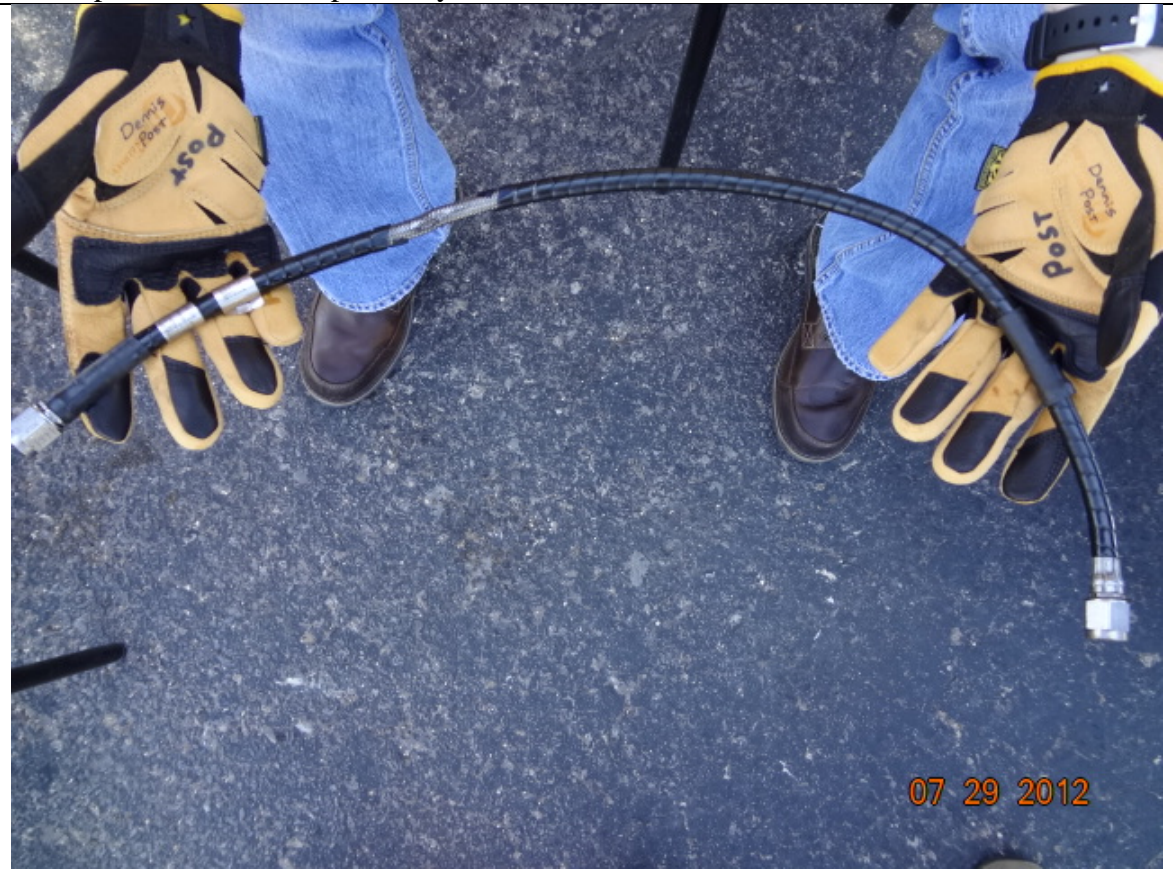
Photo 10: N379SW ruptured hydraulic line
