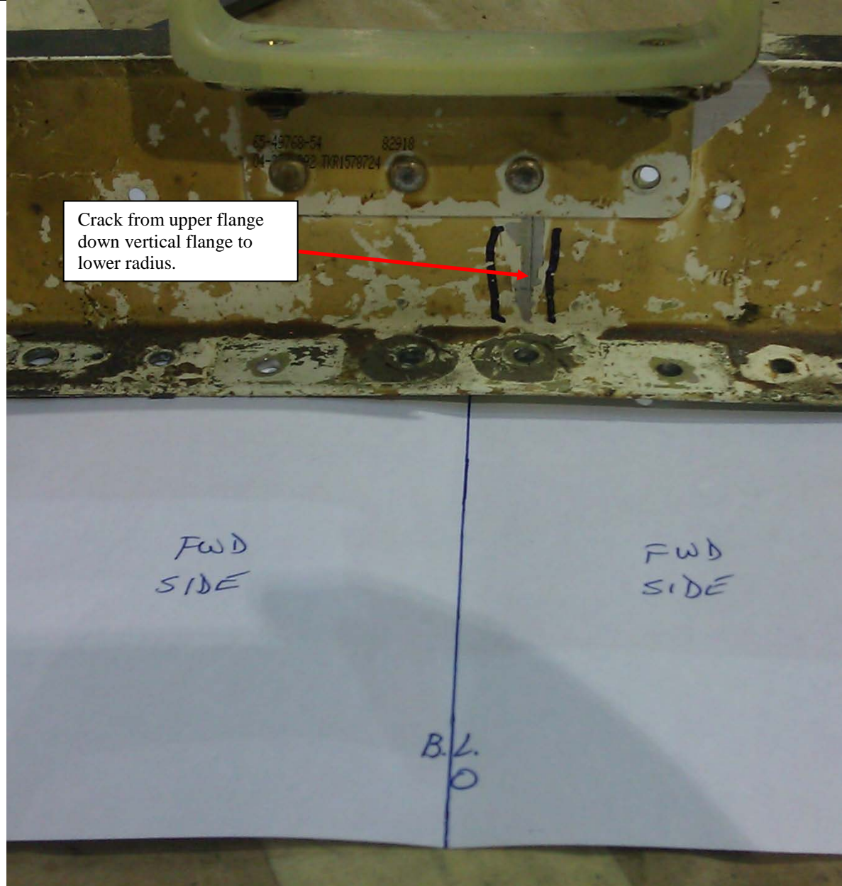
Photo 8: N379SW forward side of the 65-45819-39 lateral stiffener
