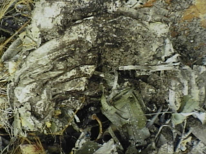
Structures/Maintenance 7 - Photo 6. Fuselage and component crushing. Note: Frayed wiring.
