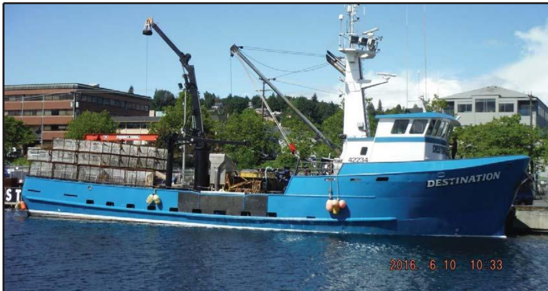
Figure (6): Starboard Profile Showing 9 Freeing Ports
