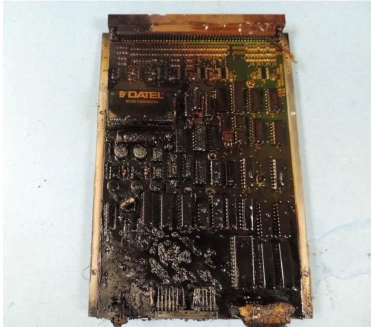
Figure 2. Bit and diagnostic card as removed from SCU.
