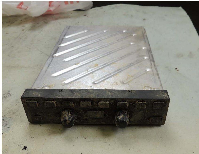
Figure 2. External damage to DFC-90 Autopilot Unit
