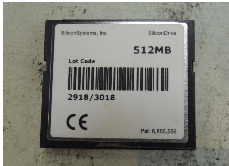
Figure 1. Undamaged CF Card from MFD
