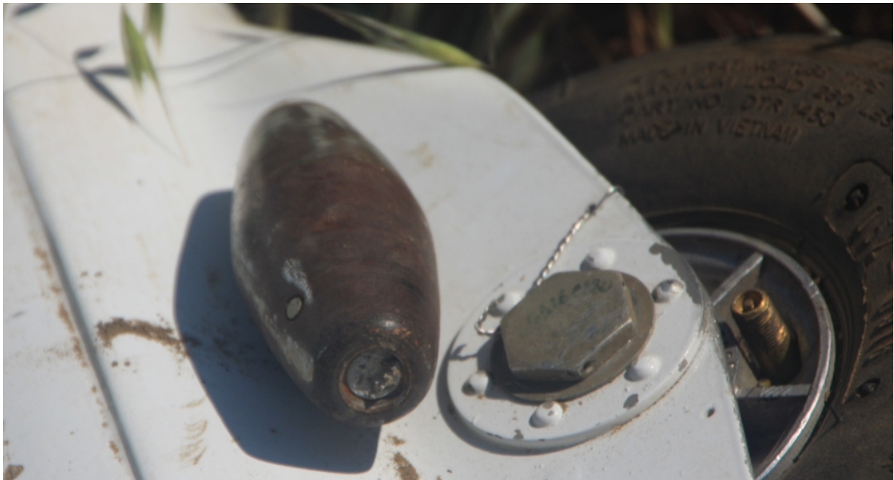
Figure 27 - Fracture-Separated Stabilator Balance Weight
