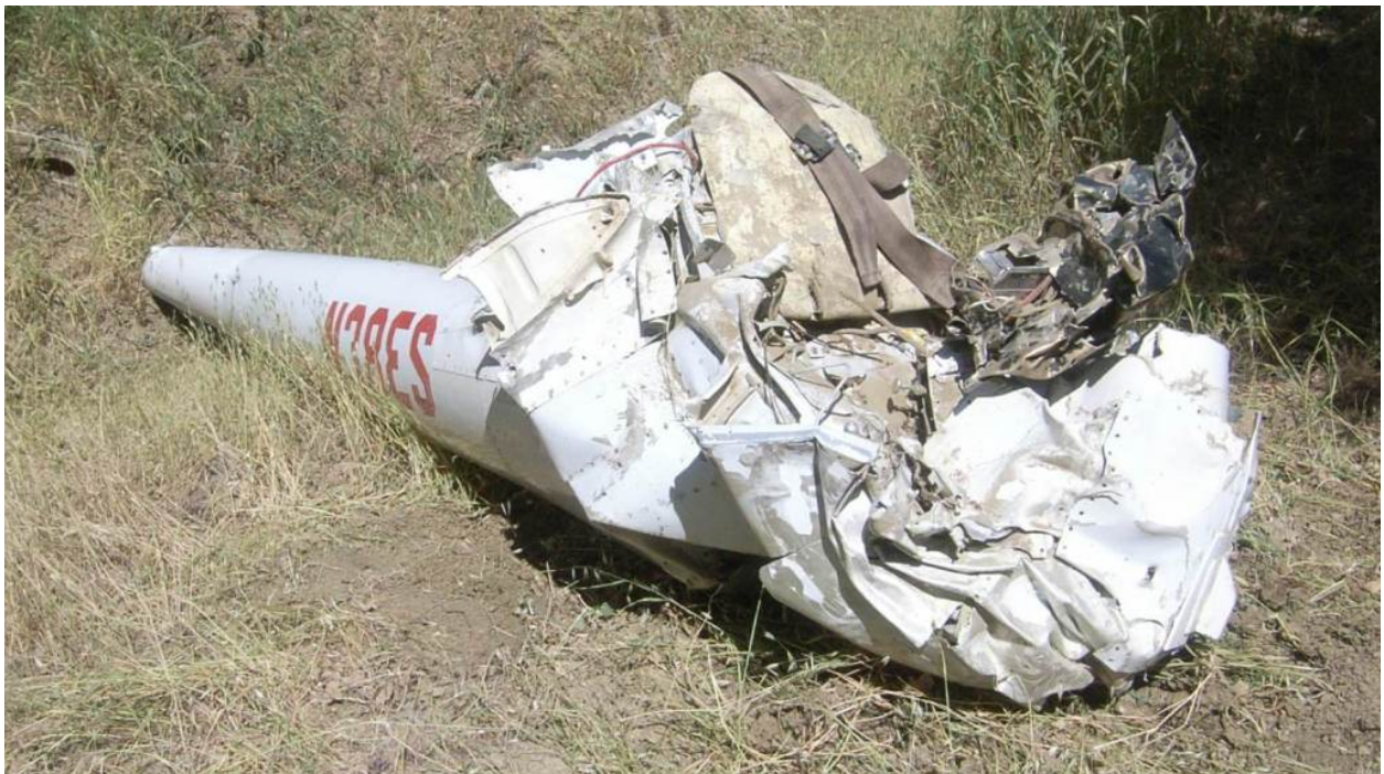
Figure 20 - Fuselage Crush (resituated for examination)
