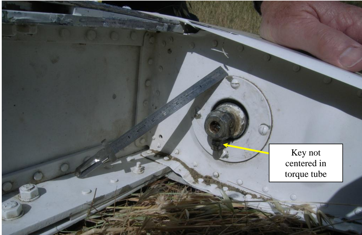
Figure 16 - Displaced Air Brake Control Indexing Key
