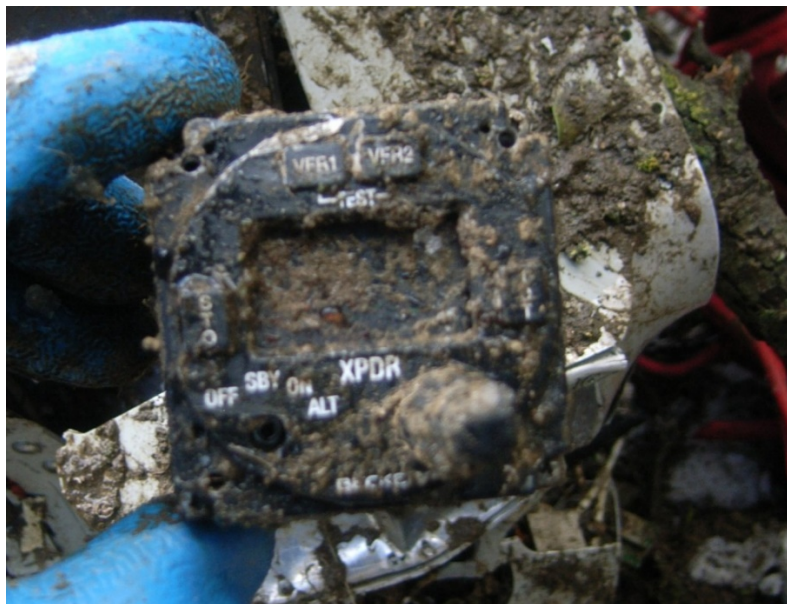
Figure 19 - Electronic Transponder Face
