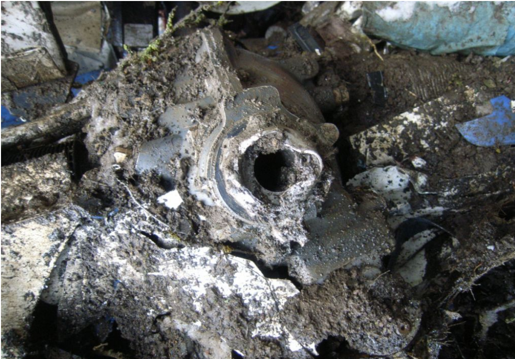
Figure 23 - Fractured Crankshaft/Propeller Hub Junction
