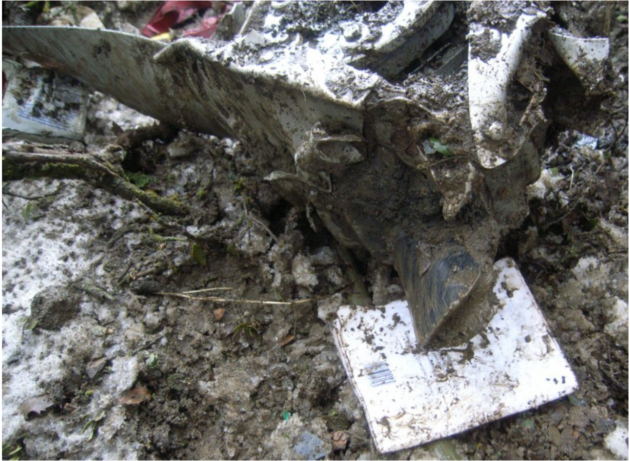
Figure 26 - Fractured Blade Root
