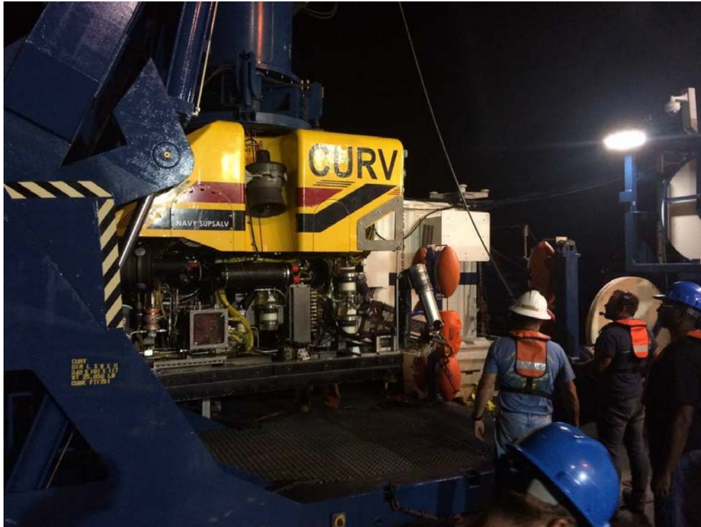
Figure C-4. CURV-21 landing on Apache deck after retrieving VDR.
