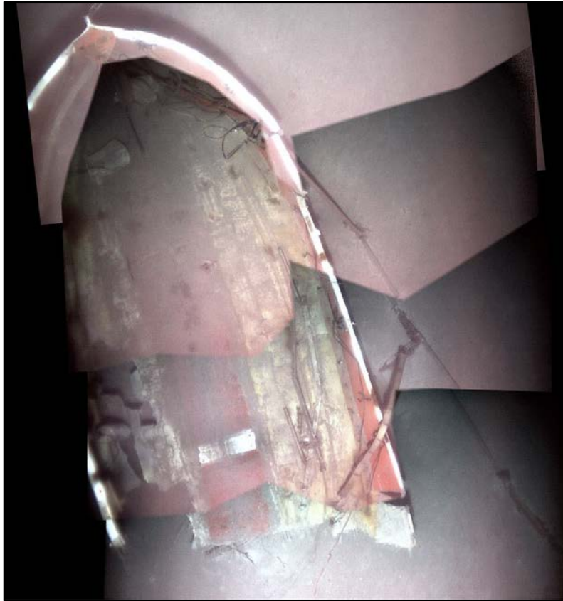
Figure 24. Photomosaic of El Faro 's port lifeboat from images taken during second search mission. Bench seats and other internals are missing. Reflective tape on top of gunwales is illuminated.
