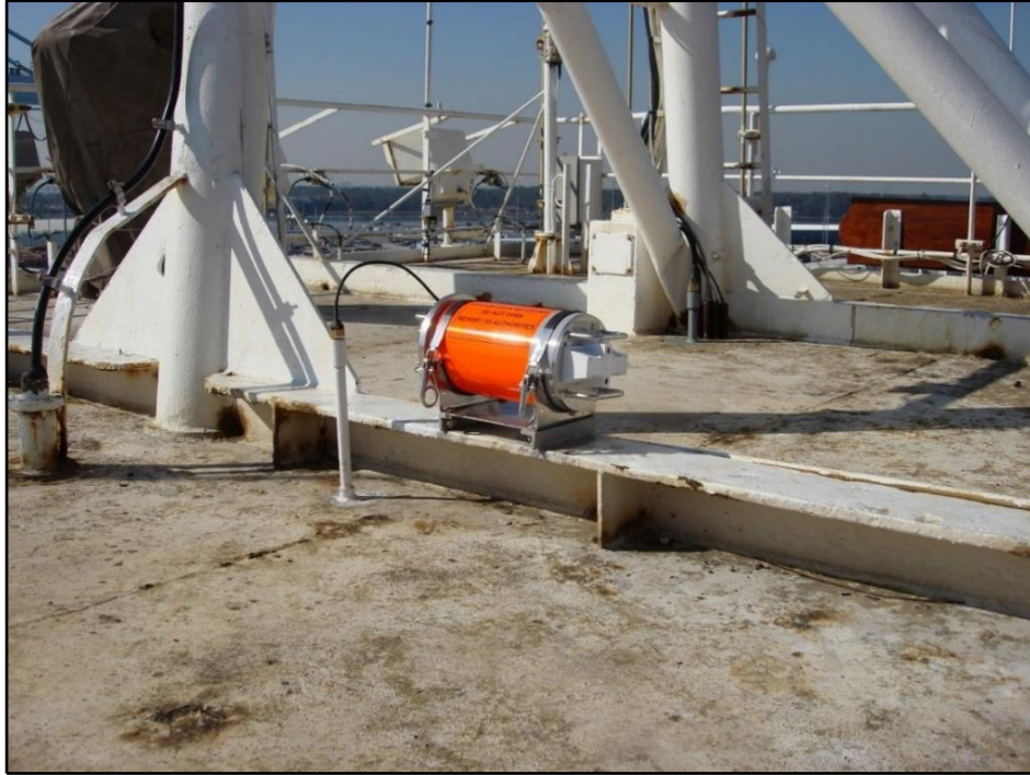
Figure 15. VDR capsule on deck above El Faro 's navigation bridge. (Radio Holland photo 80 )
