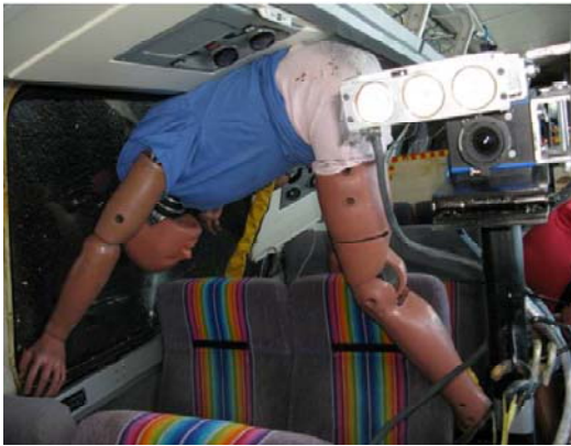
Figure 17: Post-Test View of Front Unrestrained Test Dummy (1992 MCI MC-12). The image has been rotated and flipped such that the occupant motion appears to be in the same direction as the accident vehicle's roll.
