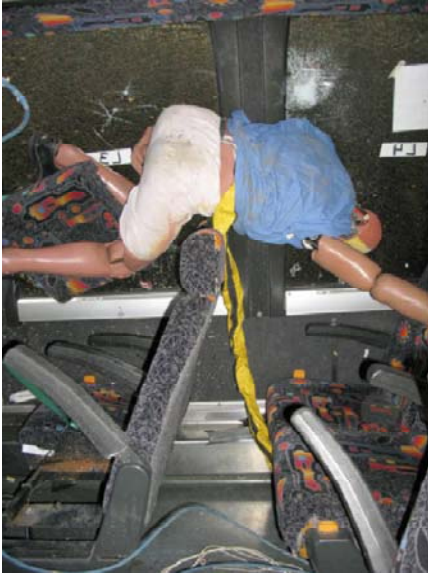
Figure 15: Post-Test View of Front Unrestrained Test Dummy (1991 PrevoSt LeMirage). The image has been rotated and flipped such that the occupant motion appears to be in the same direction as the accident vehicle's roll.
