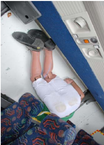
Figure 15: Post-Test View of Front Unrestrained Test Dummy (1991 PrevoSt LeMirage). The image has been rotated and flipped such that the occupant motion appears to be in the same direction as the accident vehicle's roll.
