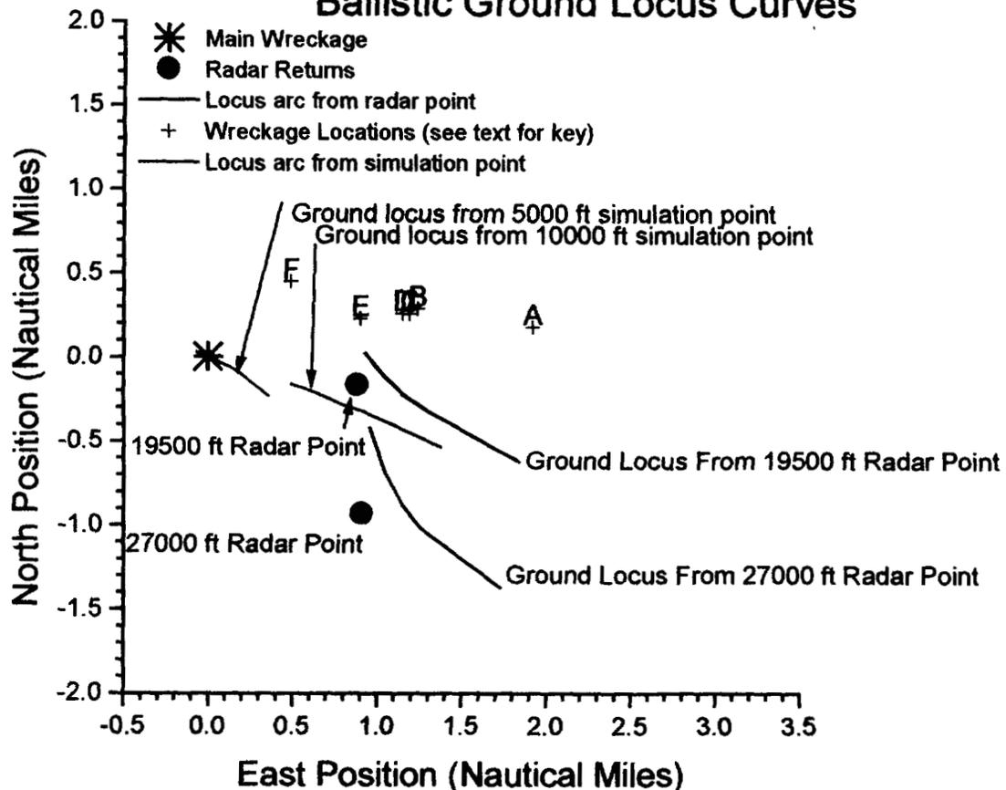
Note again that there are multiple simulations that can get from the last radar point to the crash site. An aircraft path that traveled further North between the last radar hit and the crash site would be required to produce a ground locus curve North of the crash site.
