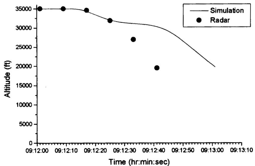
Rudder Hardover (with pilot response against the roll)
