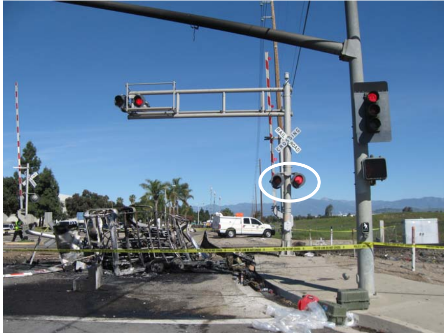
Figure 1. Photo taken, north direction, wreckage of trailer associated with utility truck after impact, & warning system devices operating after island gate knock down. The plastic covers for the LED flashers were burned on the cantilever.
