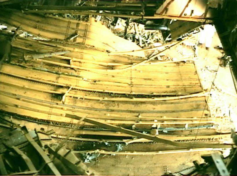
Sequencing Group 18 - Appendix B - Photo 9. View showing deformation of the lower skin.
