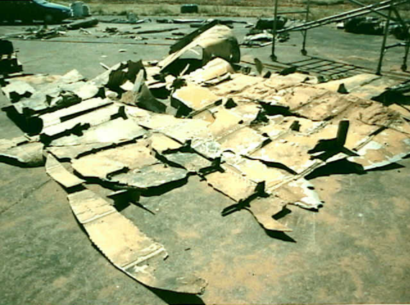
Sequencing Group 18 - Appendix B - Photo 8. View showing deformation of the upper skin.
