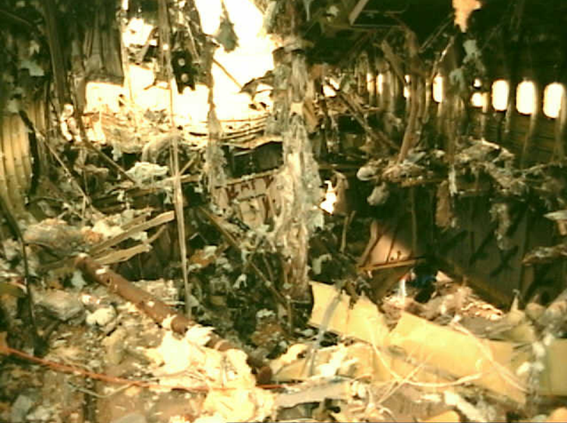
Sequencing Group 18 - Appendix B - Photo 6. View showing damage of wing center tank after explosion.
