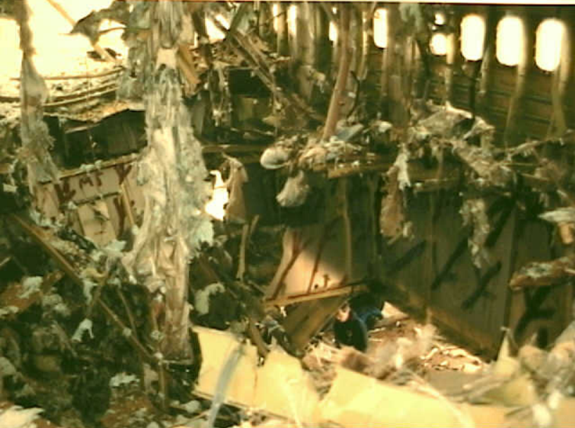
Sequencing Group 18 - Appendix B - Photo 18. View showing damage to LSOB rib.
