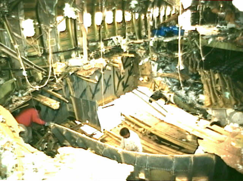
Sequencing Group 18 - Appendix B - Photo 17. View showing damage to RSOB rib.
