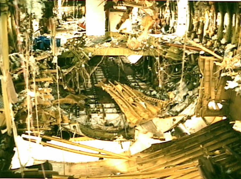
Sequencing Group 18 - Appendix B - Photo 10. View showing sections of front spar pushed forward.
