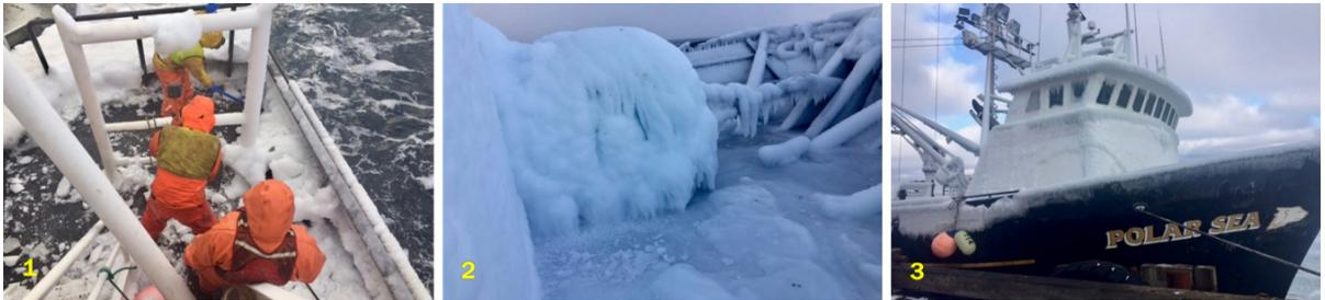
Ice accumulation on a vessel operating near the capsized vessel that was lost with all hands in the Bering Sea on February 11, 2017. (1, 2, and 3) *Polar Sea*: ice covers the decks and anchor chain during the vessel's transit to St. Paul Island on February 10 and remains on the wheelhouse while it was docked at the island the following day.
