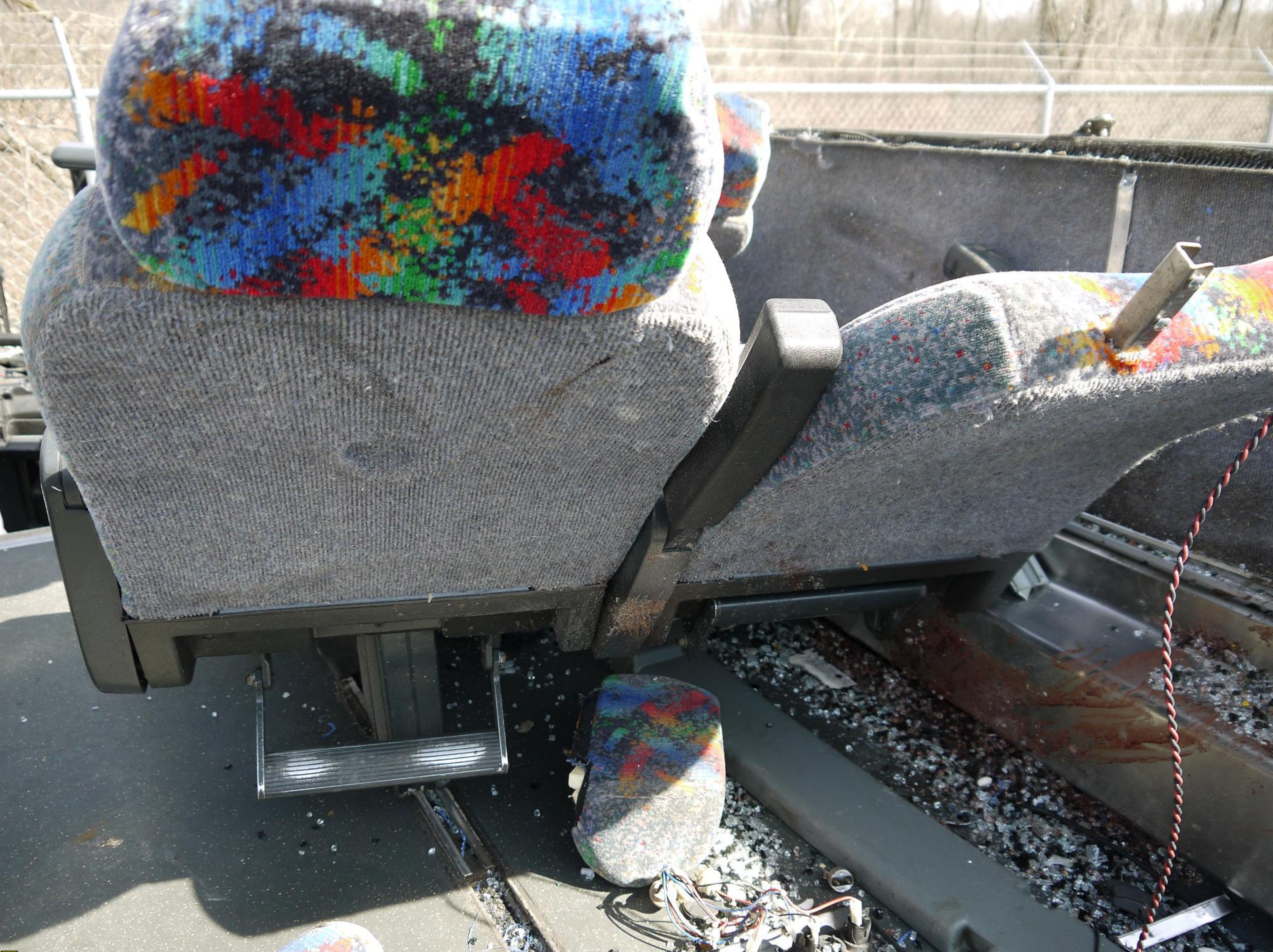
Photo 8 View of Row 2 Passenger Side with Occupant Impact Mark
