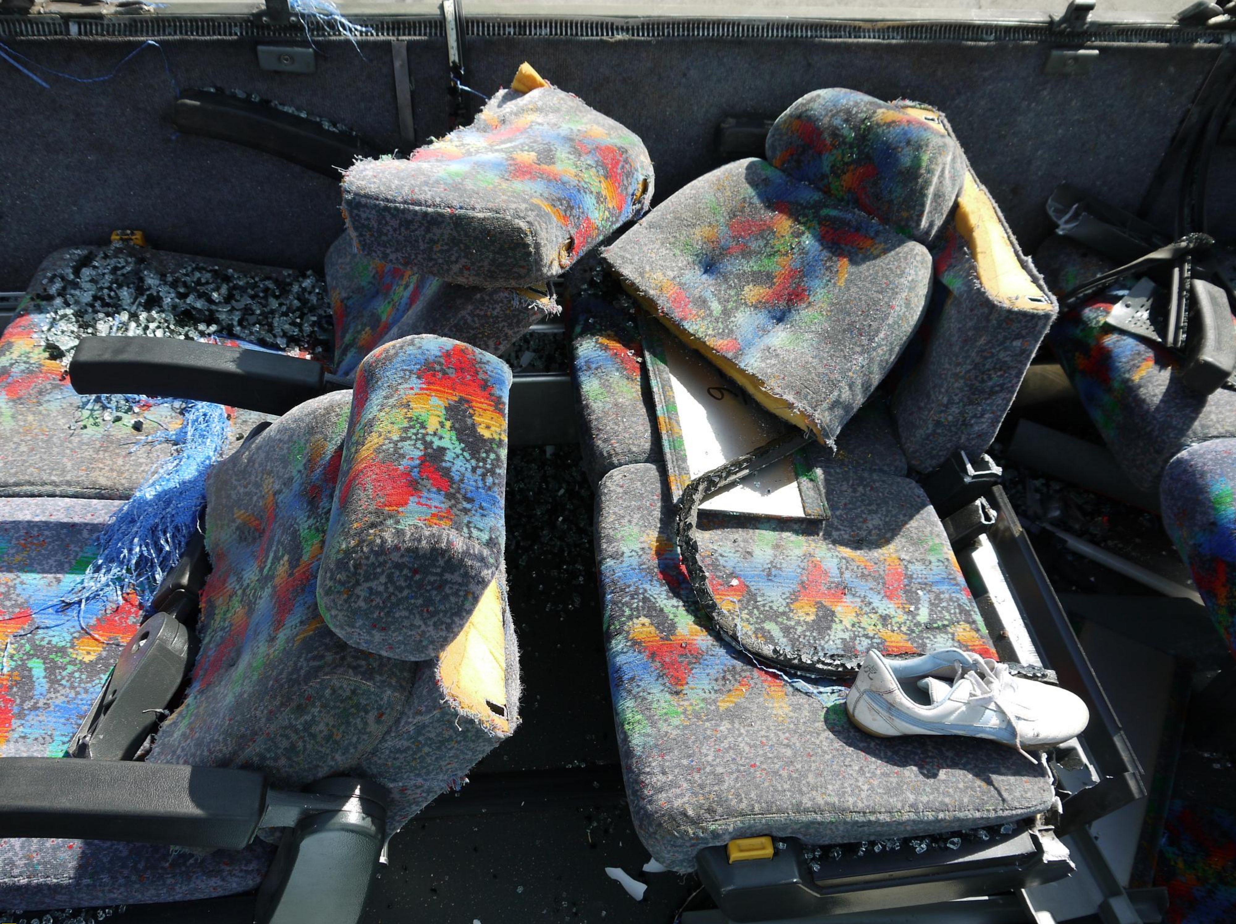
Photo 6 View of Seatbacks Cut During Extrication
