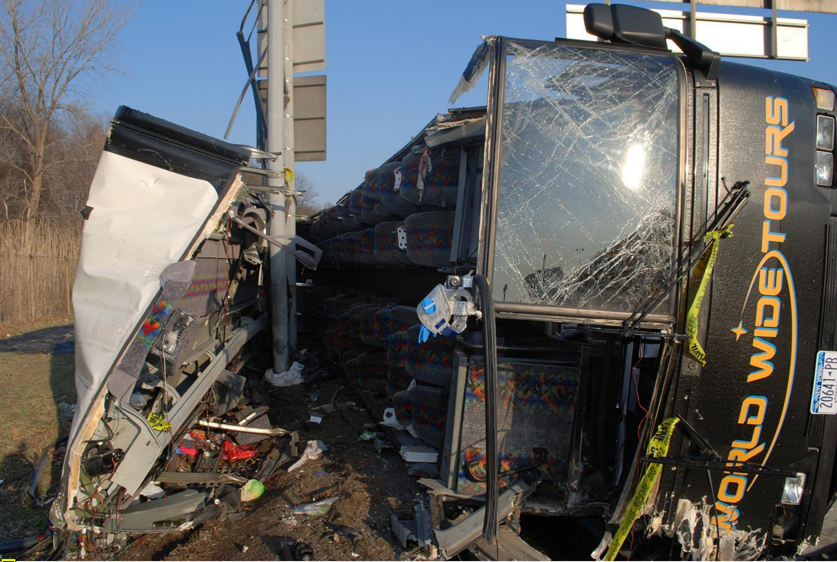
Photo 5 Front and Interior View with Stanchion Intrusion and Parcel Rack Frame
