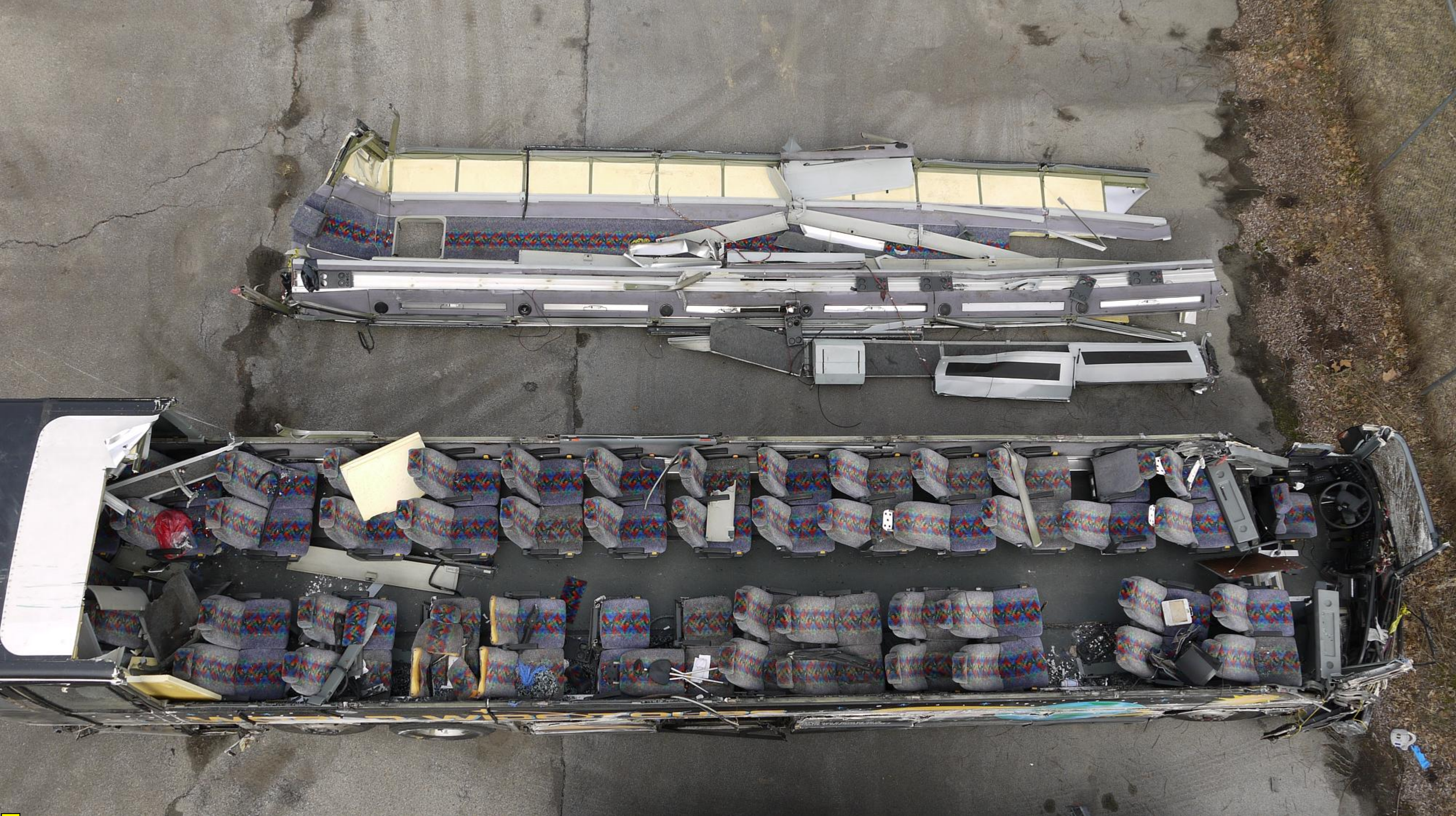
Photo 11 Aerial View of Bus Interior and Removed Inverted Roof
