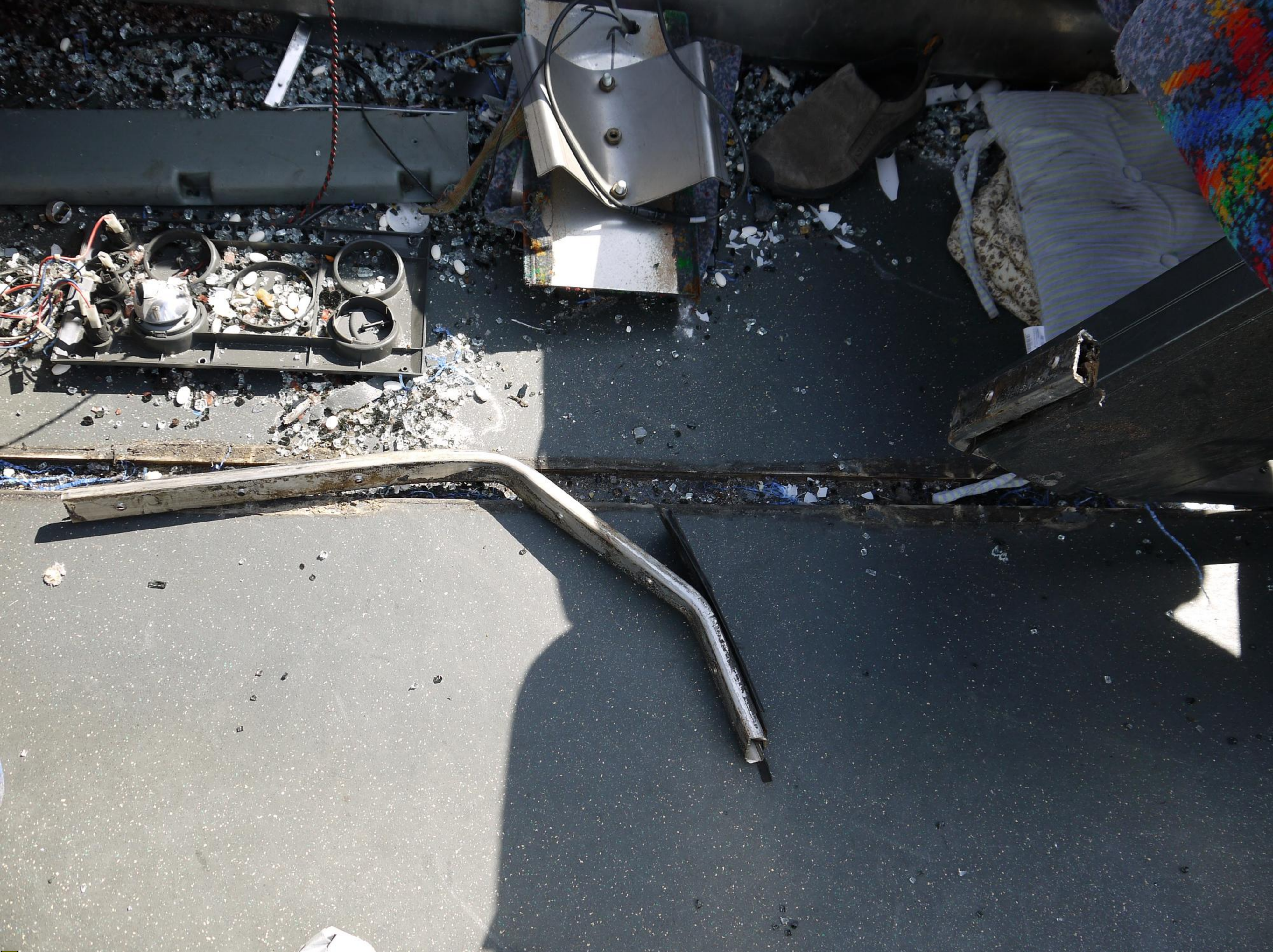
Photo 10 View of Row 3 and 4 Passenger Side Seat Track and Video Monitor Bracket
