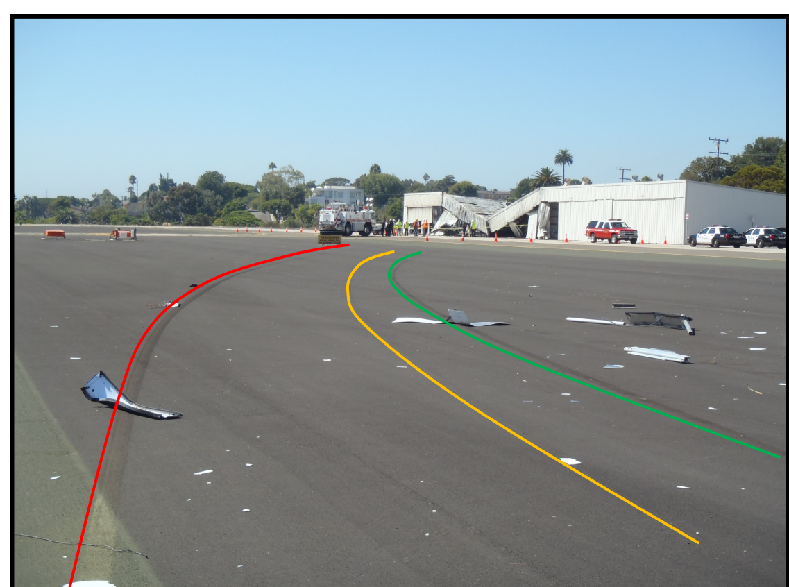
(F2) Black transfer marks for all tires leading to the main wreckage
