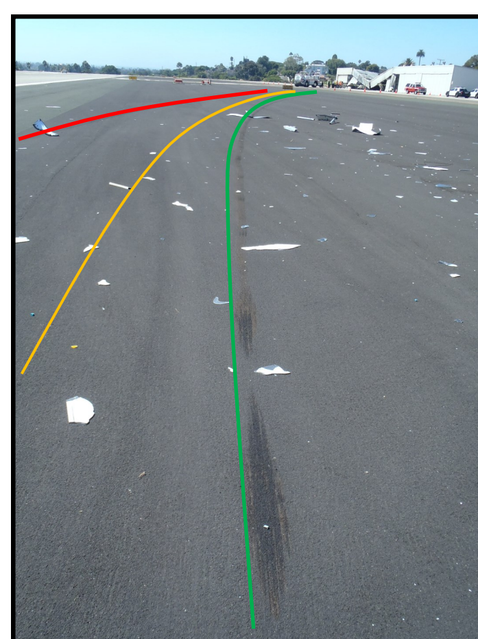
(F1) Black transfer marks, each with 5 treads of the right main landing gear tire, with scuff marks to the runway corresponding to the nose and left main landing gear tires.
