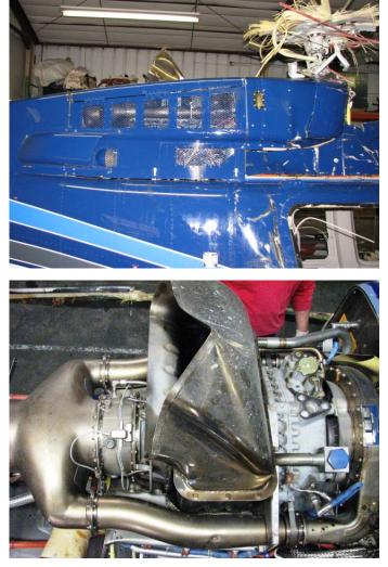
thermal degradation. There was no impact damage, metal splatter or evidence of rubbing around the air shrouds.
