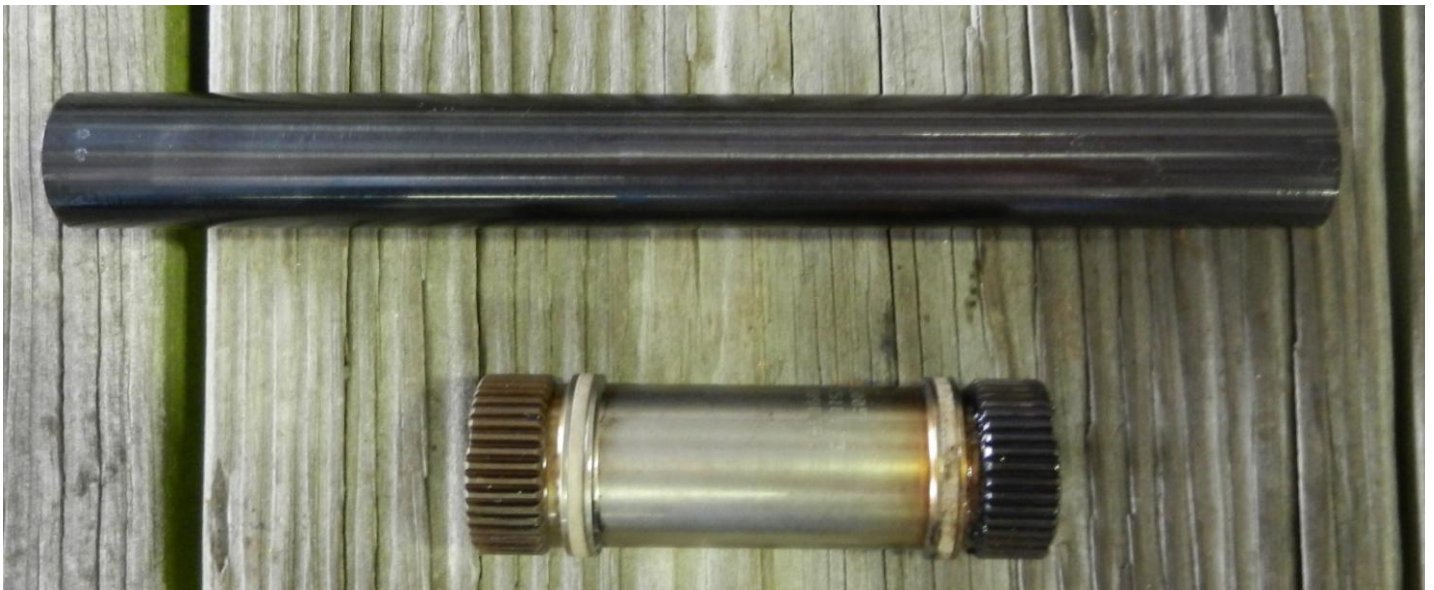
Power Turbine To Pinion Gear Coupling And Turbine To Compressor Coupling
