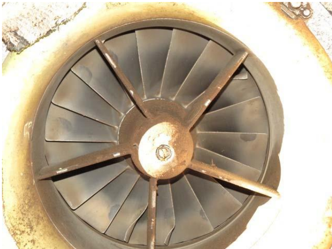
Compressor Inlet / Impeller
