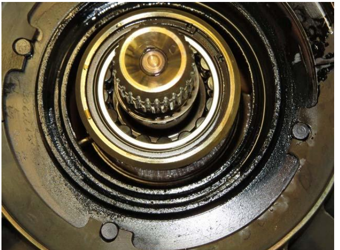
#6 Bearing in Position
