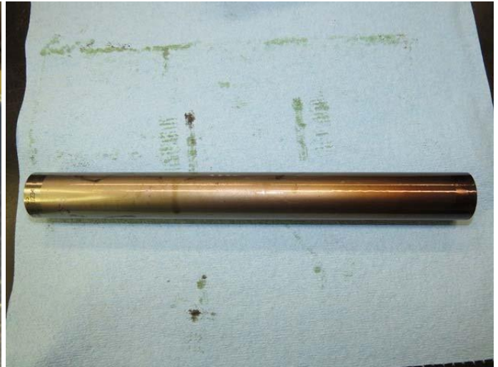
Turbine to Compressor Coupling
