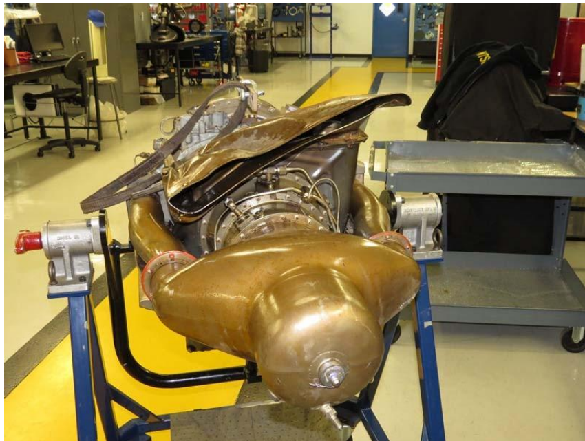
Exhaust Collector Support Damage
