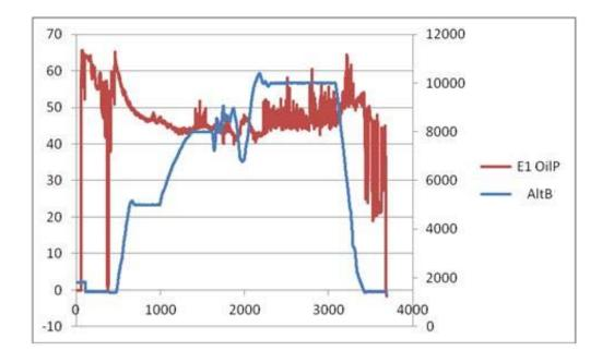
Several potential causes were explored for this issue and in the end, two causes were identified as contributing to the erratic behavior. Both of those causes were due to connectors. The first was baffle connector and the second was the connector at the sensor.
