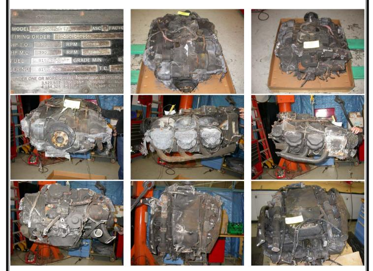
**AIRFRAME PARTS RETURNED WITH ENGINE:** Portions of cooling baffles, propeller de-ice brush block assembly and slip-ring assembly, propeller governor, vacuum pump, vacuum system filter and associated hardware, tachometer generator, fuel flow transducer and portions of wiring harnesses, hoses, tubing and control cables.
