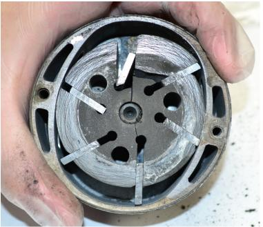
• Visual inspection of cavity shows signs of deformation due to impact.
