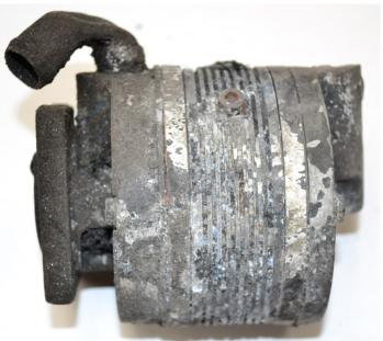
• Visual inspection of the article drive end showed that the external drive gear and shear coupler are damaged beyond recognitions due to heat damage.
