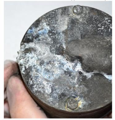
• Visual inspection of front end shows deformation due to impact.
