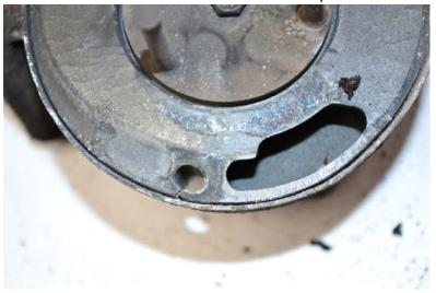
• Visual inspection of vacuum pump shows rotor cracked and one vane chipped (Vane later identified as Vane 5 was chipped).
