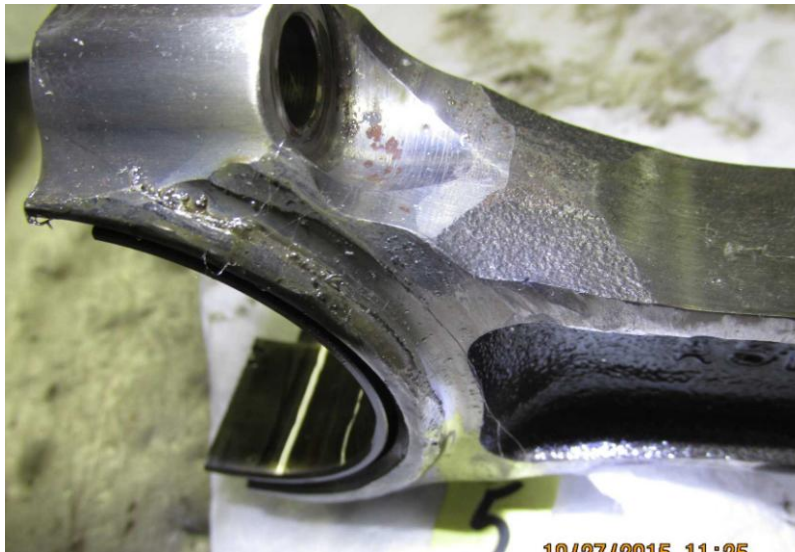
Figure 13. The #5 connecting rod's side faces were worn from contact with the crankshaft's #8 cheek thrust face, adjacent to the #5 crankpin journal. This most likely occurred during fracture, as the crankshaft's fatigue crack opening displacement grew progressively larger.
