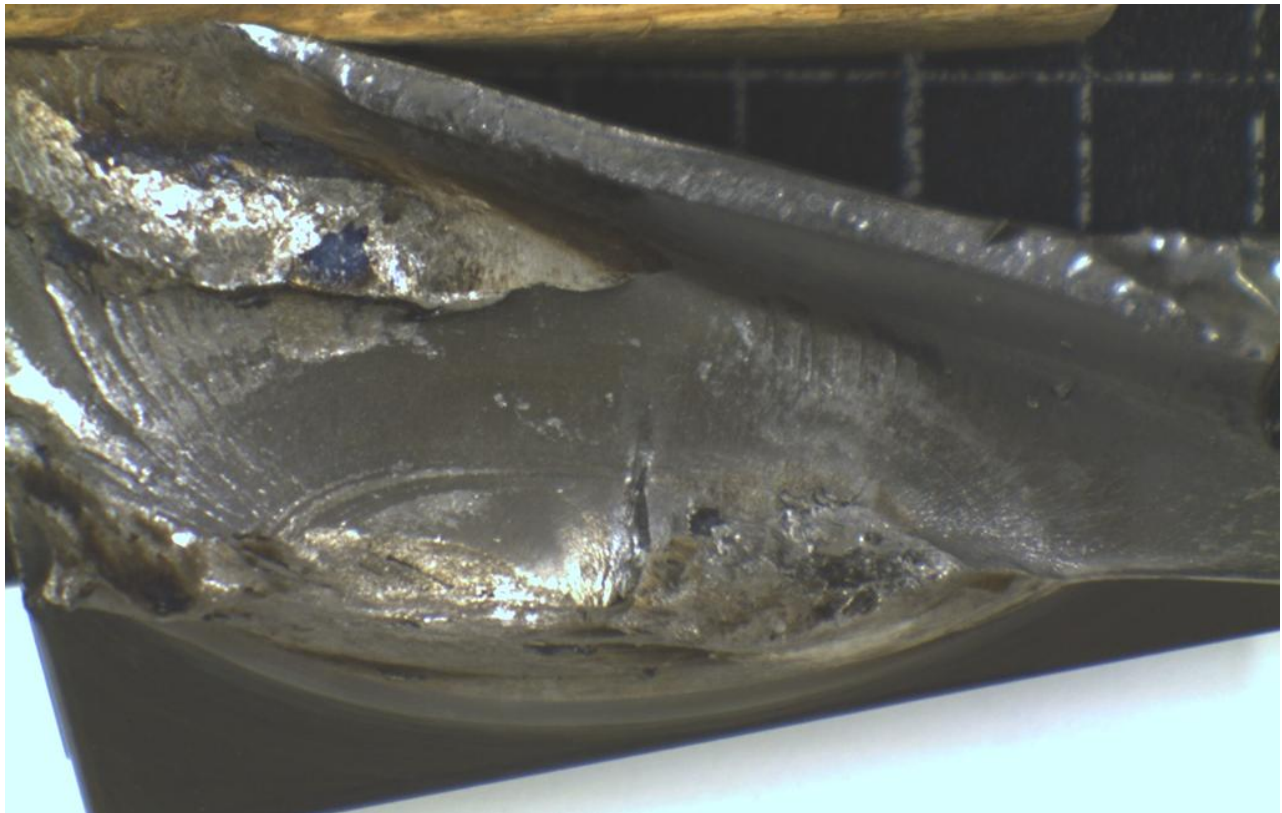
Figure 32. Crankshaft fracture surface, displaying beach marks indicating fatigue crack initiation near the rear crankpin journal fillet radius, from at least one and possibly two or three origin sites. See Figure 33 for closer views of the origin area. White gridlines = 1 cm.
