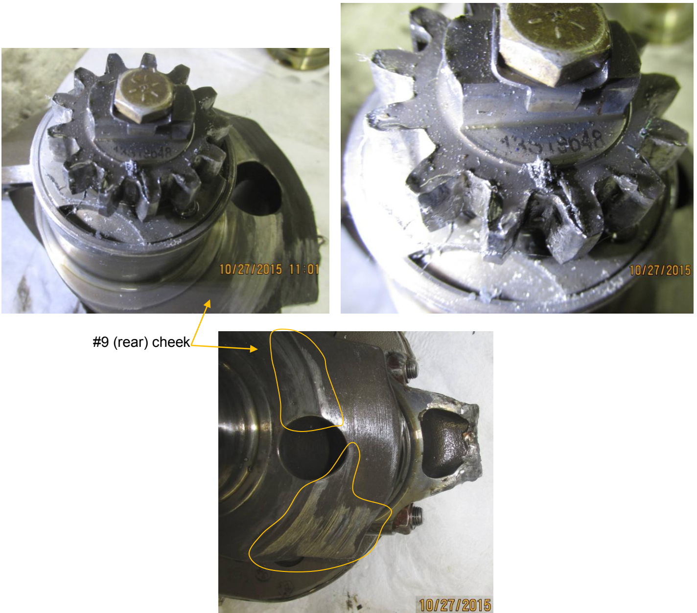
Figure 9. The rear end of the crankshaft, with gear still installed (top photos). Note severely damaged gear teeth, most likely caused by the impact with the ground. Also note, gear bolt and bolt locking plate both still installed and undamaged. Also note, in left and bottom photos, the rear side of the #9 cheek exhibits wear and scoring marks (circled), from contacting the crankcase saddle during final fracture. Broken #6 connecting rod also visible in bottom photo, with connecting rod bolts and nuts still attached tightly.
