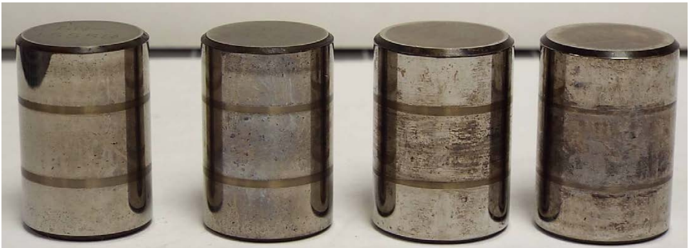
Figure 31. Counterweight rollers that were installed in bores A1, A2, B1, and B2 (left to right). Note, the crack grew into the B2 lug, releasing the crankshaft's bushing, and causing some wear on the B2 and the B1 rollers. Otherwise, all four rollers were in good condition.
