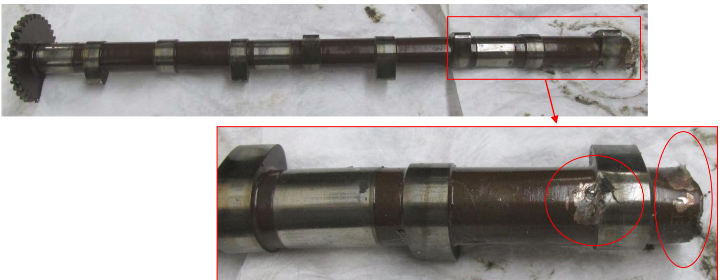
Figure 21. Broken camshaft, with hard impacts visible in several locations (circled).
