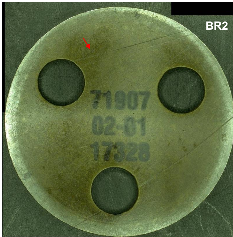
Figure 30. Counterweight washer BR2 displayed cracking on its outward face (arrows).
