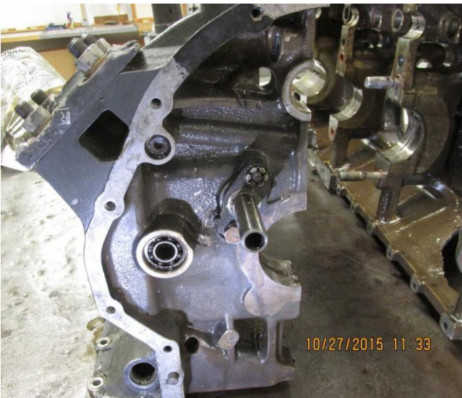
Figure 17. Rear view of the left crankcase half (left). At right, a view showing the engine mount bracket on this side was also broken ( right, circled ).
