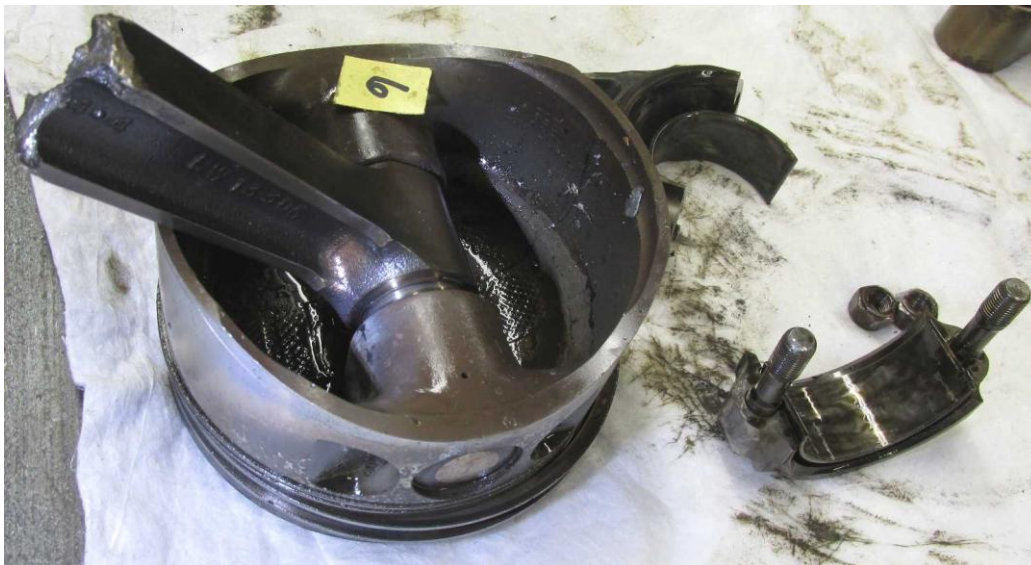
Figure 14. The #6 connecting rod was fractured through the web section, near the crankpin bore end. This fracture surface was very badly damaged from post-fracture contacts.
