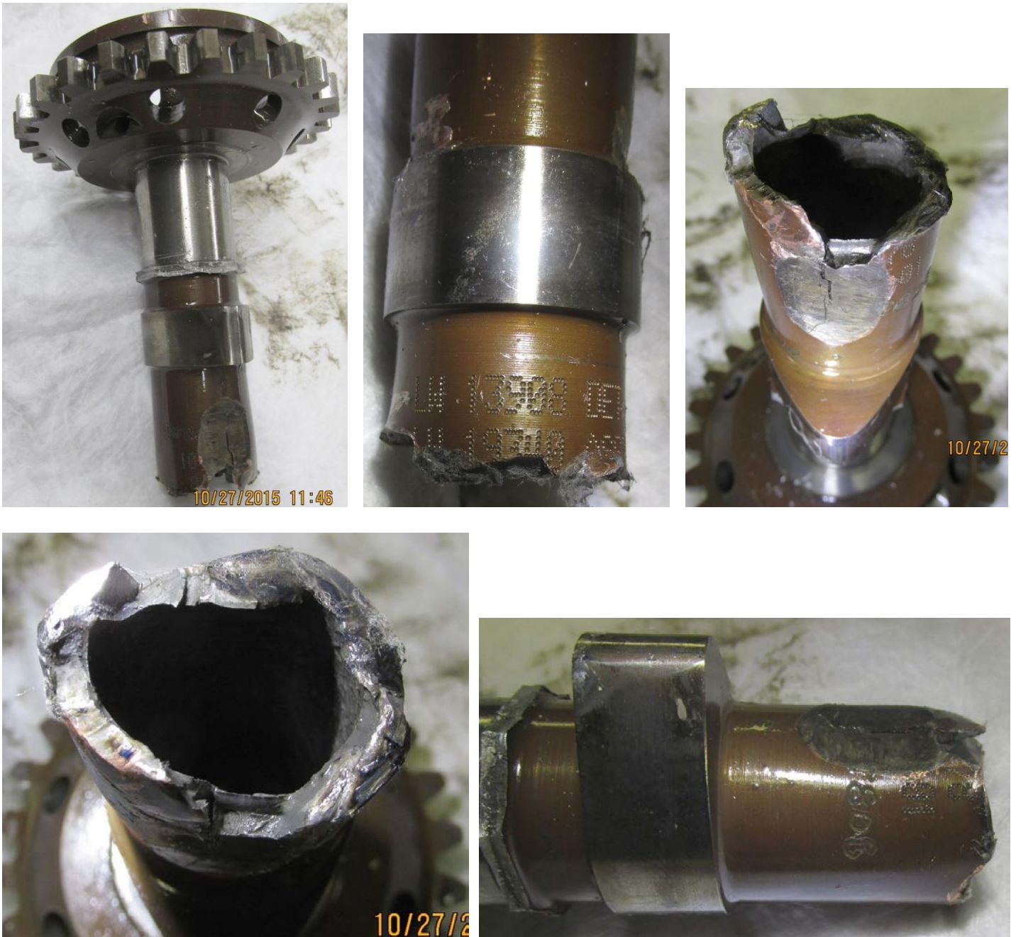
Figure 22. Mating piece of the broken camshaft, also exhibited several hard contact marks. Shaft was broken through the non-carburized region between the #5/#6 intake and the #6 exhaust camlobes. Fracture surface was completely smashed and could not be evaluated, but evidence indicates fracture was most likely caused by hard impacts from other engine components.
