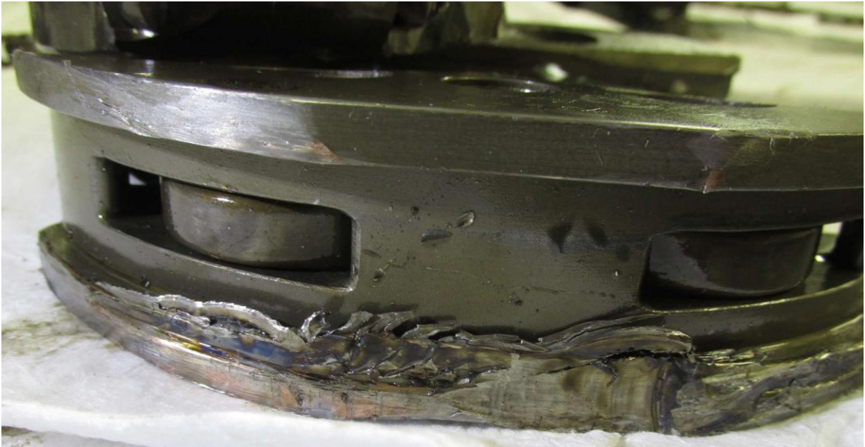
Figure 11. The outer surfaces of the A counterweight body, still attached to crankshaft. Note severe damage from contact with other engine components during final stages of fracture and/or impact with the ground.
