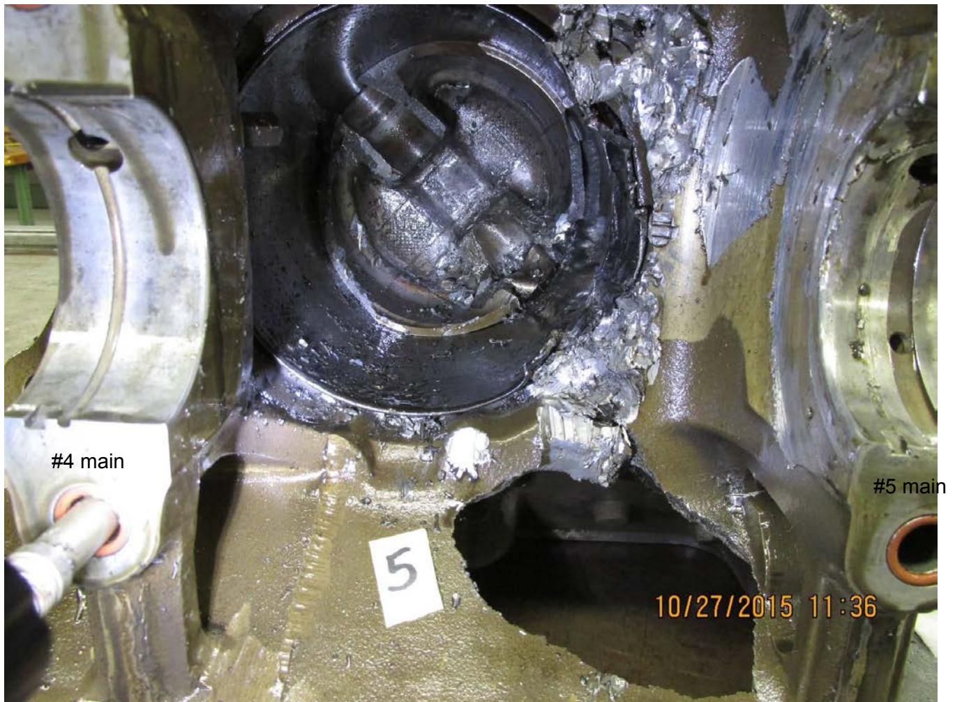
Figure 20. Severely damaged crankcase walls in the vicinity of the #5 cylinder barrel. Note damage to the #5 rear main journal support saddle (right side of photo), caused by hard contact with the crankshaft's #9 cheek. Also note the #5 piston stuck inside the cylinder, twisted from its normal installed orientation, and with several chunks ripped free by the connecting rod and piston pin (the #5 connecting rod was bent, but not broken, and still had the piston attached – see Figures 1, 2, and 12).
