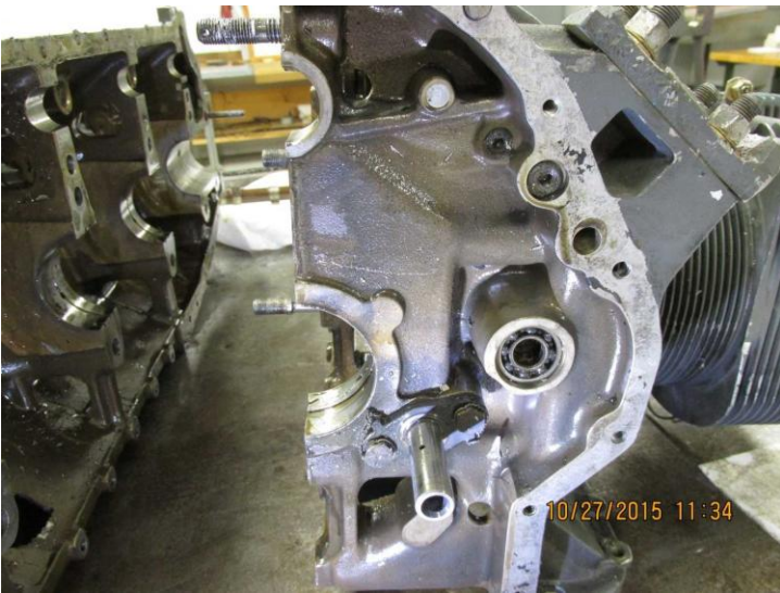
Figure 16. Rear view of the right crankcase half, and a view from different perspective, showing the broken engine mount bracket ( right, circled ).
