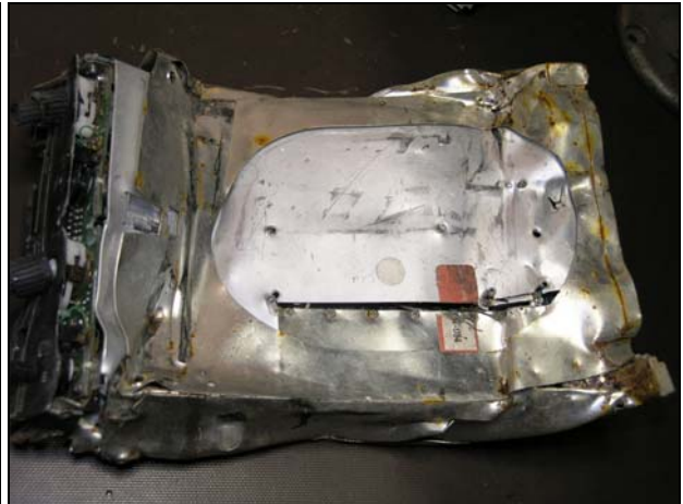
KX155 impact damaged – top and bottom views exhibit crushing damage
