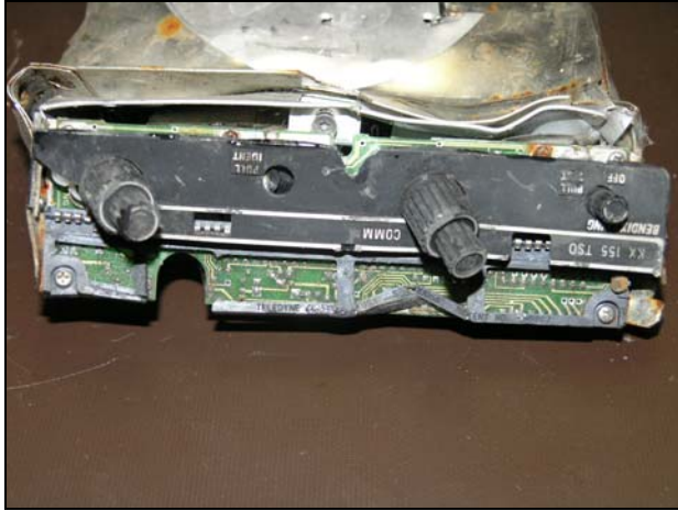
Front bezel partially missing
