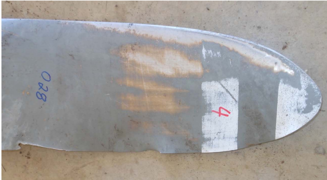
Photo #14 – Blade #4 chordwise/rotational scoring on camber side
