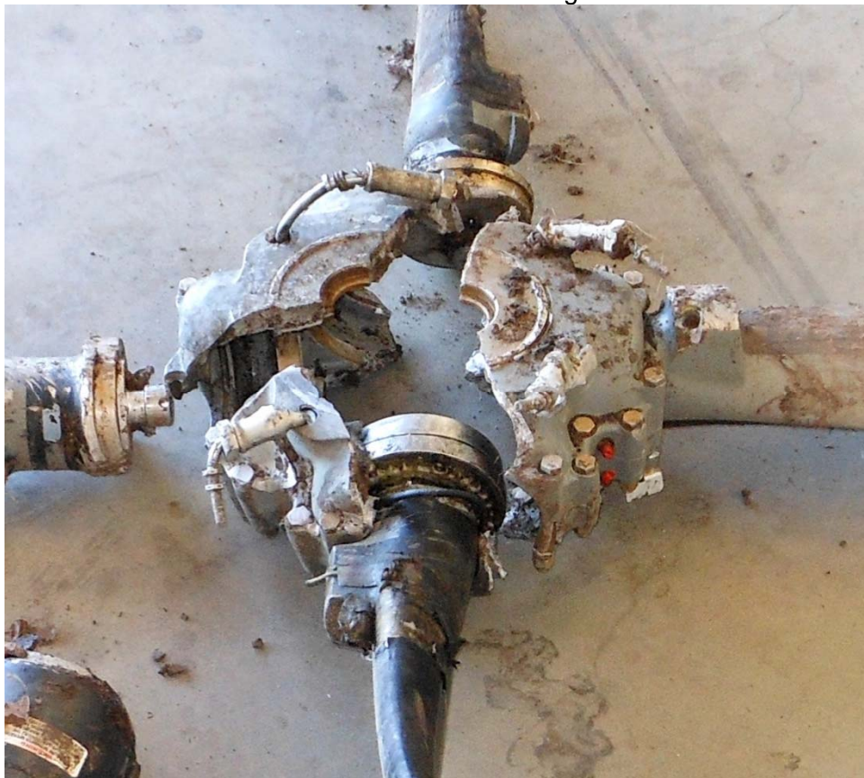
Photo #5 – Fractured hub fragments
