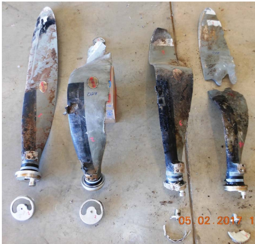
Photo #7 – Blades camber side shank view
