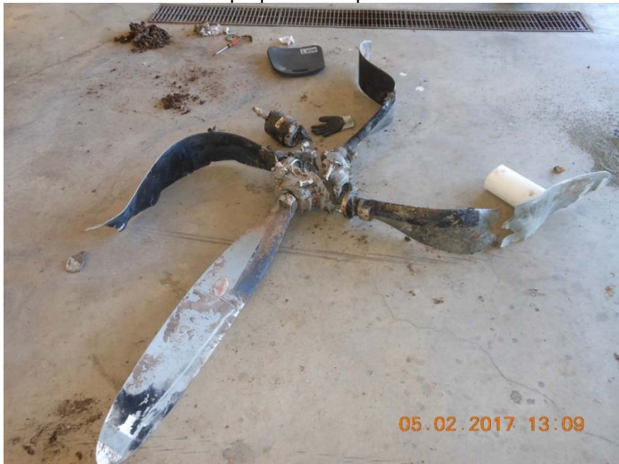
Photo #3 – Main propeller components as-recovered
