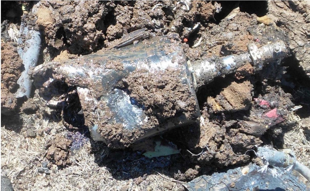
Photo #4 – Hydraulic Unit as recovered
