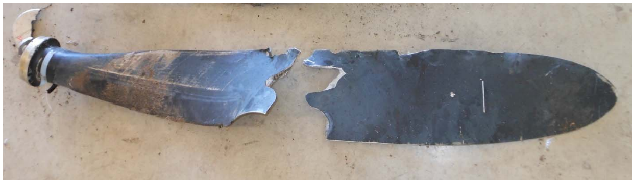
Photo #13 – Blade #4 fracture
