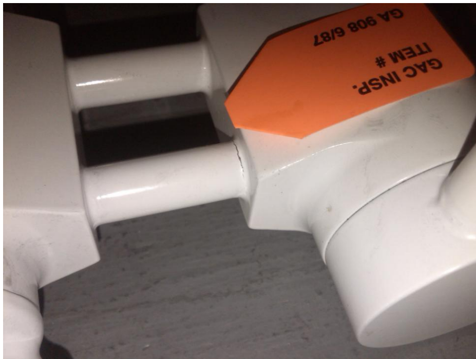
FIGURE 1 FAILED SWIVEL S/N 0689
