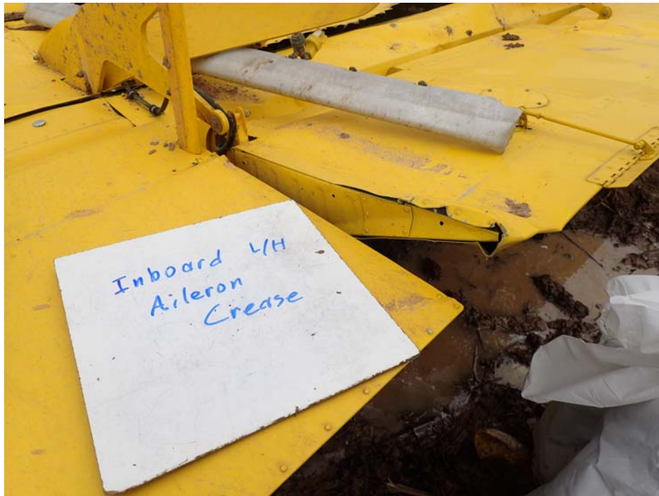
Crease on Inboard Lefthand Aileron
