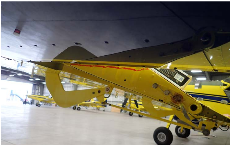
Deflection of Lefthand Aileron on Exemplar AT-802A
