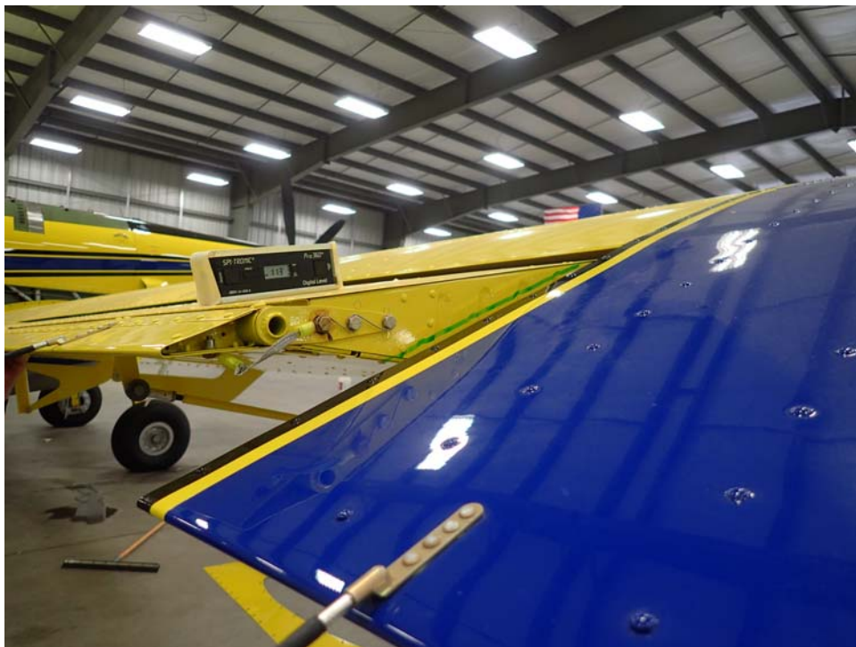
Deflection of Righthand Aileron on Exemplar AT-802A
