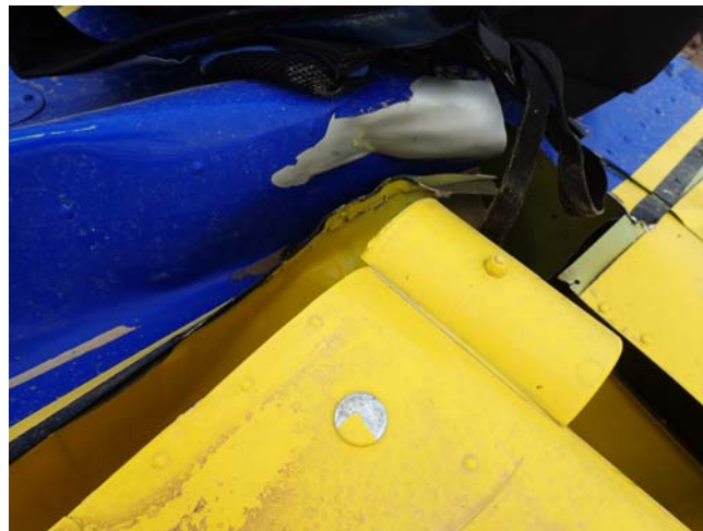
Contact of Righthand Aileron Counterweight with Trailing Edge Skin
