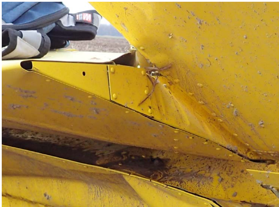
Crease on Inboard Righthand Aileron
