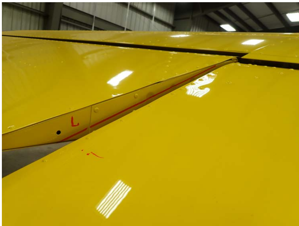
Deflection of Lefthand Aileron on Exemplar AT-802A
