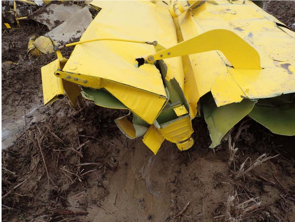
Crease on Outboard Lefthand Aileron
