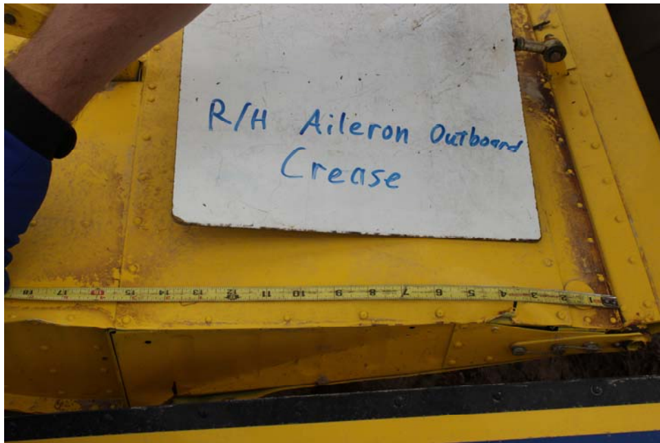
Crease on Outboard Righthand Aileron
