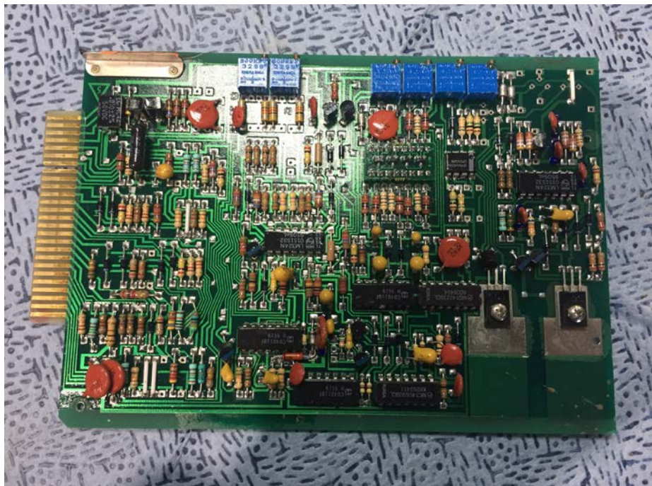
KC 295 Adapter board, P/N 065-5009-82, Mods 8, 9. This is the correct Adapter board for the 58 Baron.
