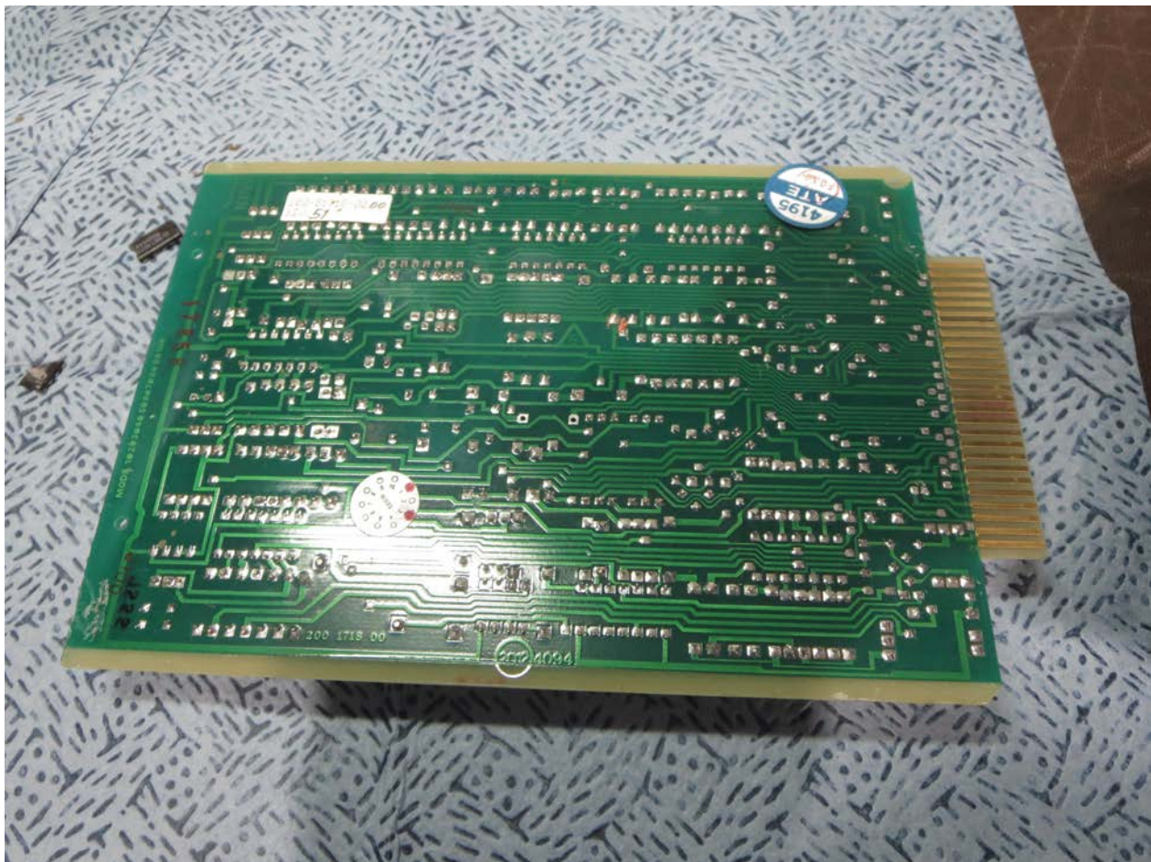
KC 295 Pitch board: contains two chipped capacitors – no other damage noted and testable
