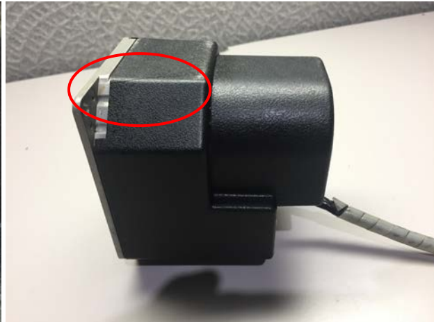
KS 272A – cover cracked
