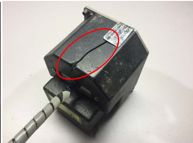
KS 271A – cover cracked/broken
