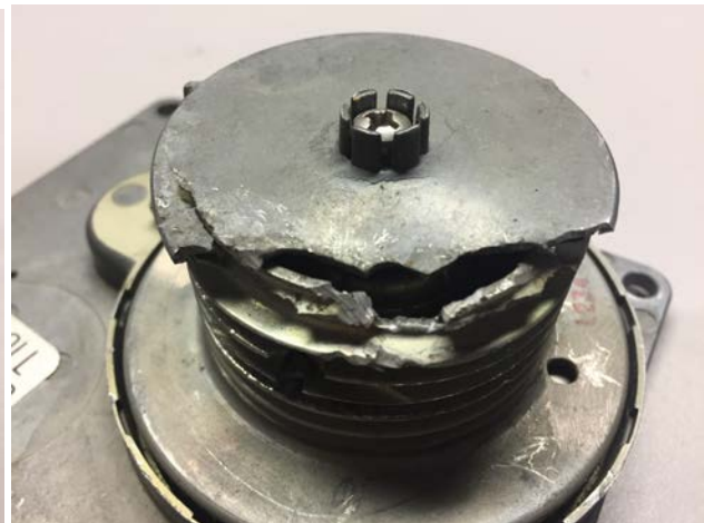
KM 275 – capstan impact damaged
