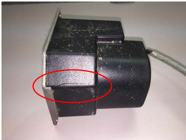
KS 271A – cover cracked
