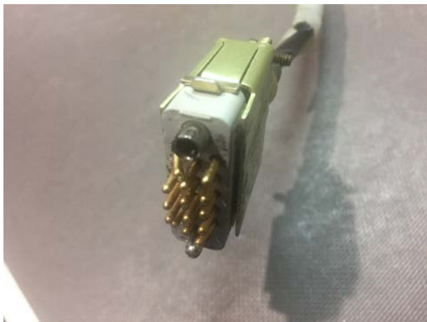
KS 271A – bent connector pins
