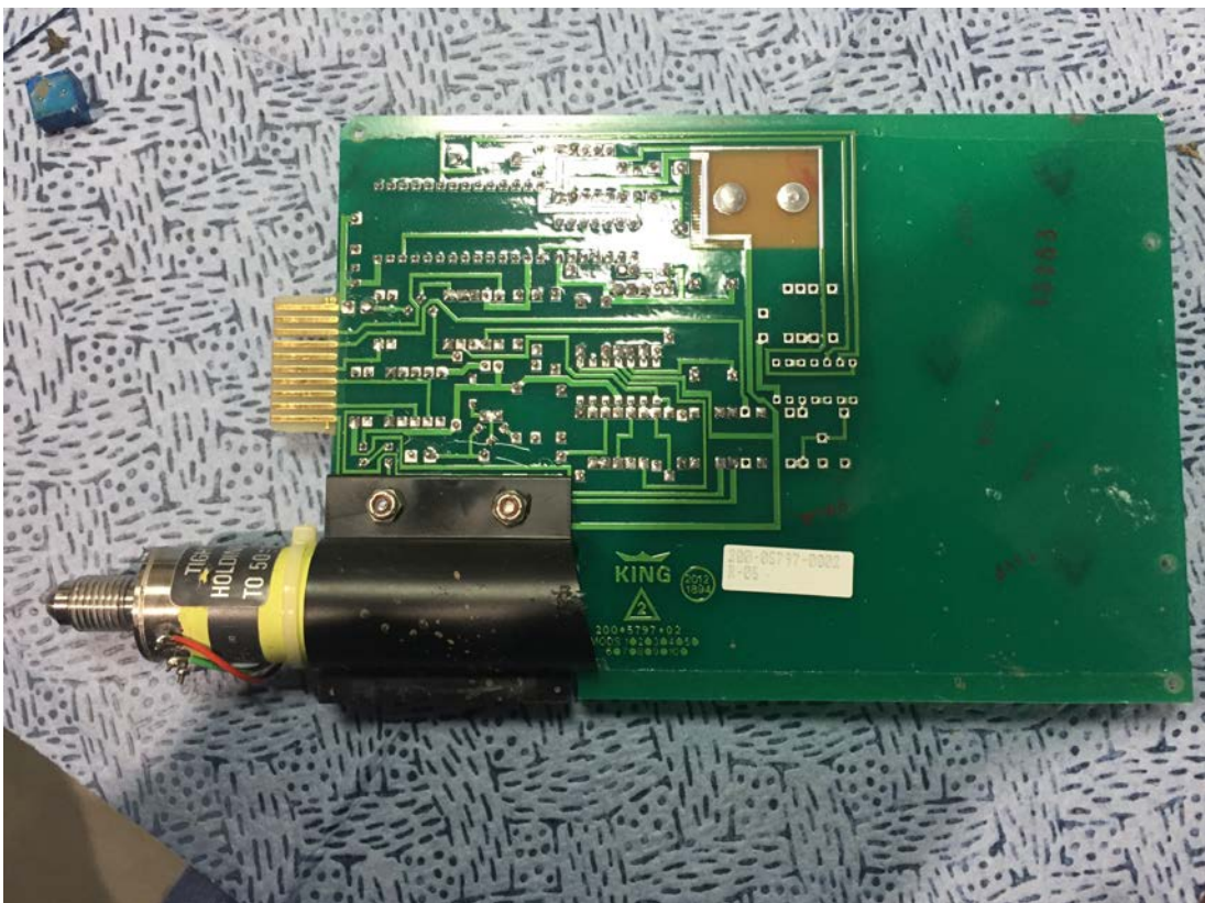
KC 295 Altitude board – no impact damage detected
