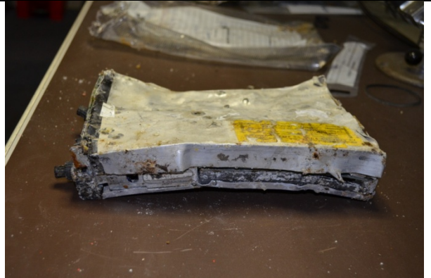
Crush damage to KX155 NTSB # 1265001
