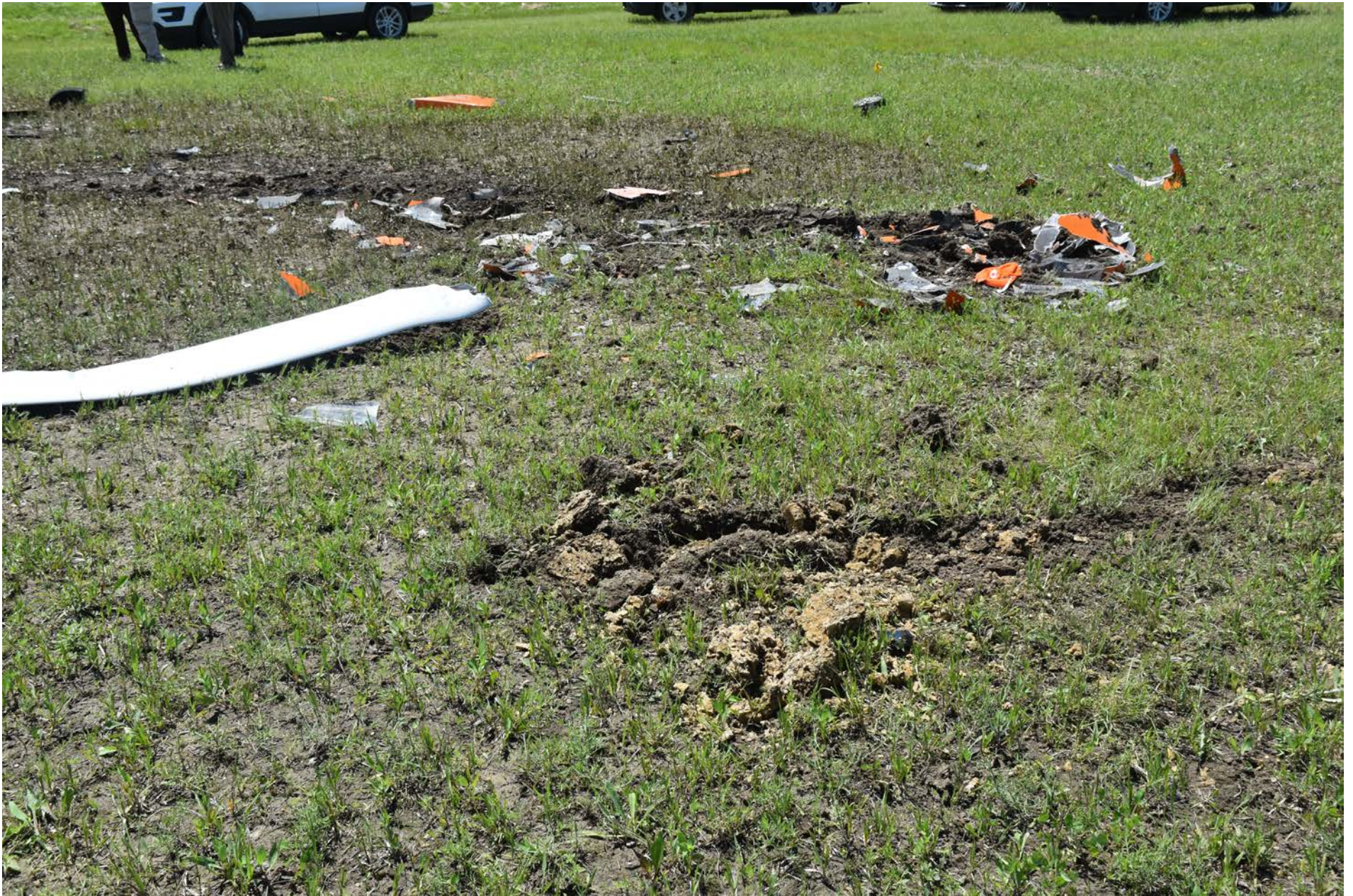
Photo 4 – Bent main rotor blades and the ground scar left when it struck the ground. Note midspan bending.
