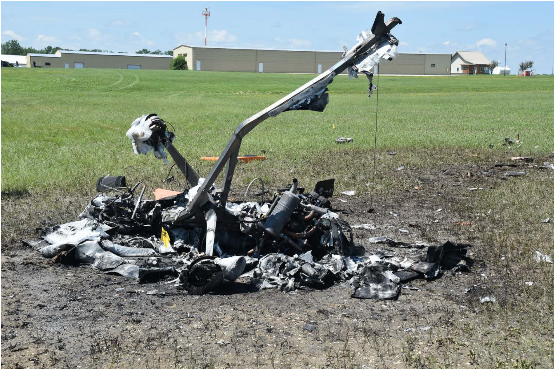
Photo 5 – View to the north. Landing gear and tailboom frame are shown.
