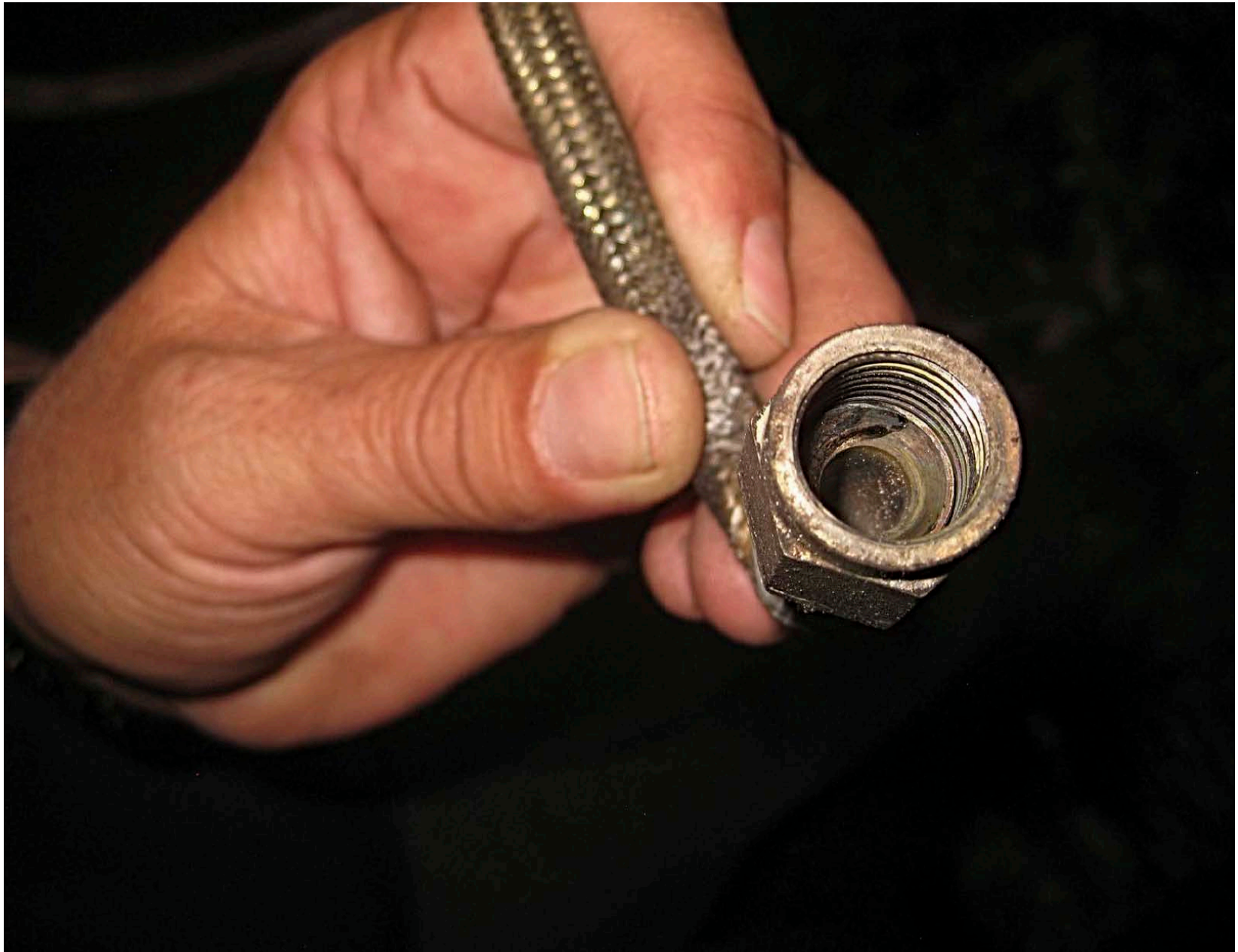
Photo 17 - Fuel pump discharge line. Note carbon deposits.
