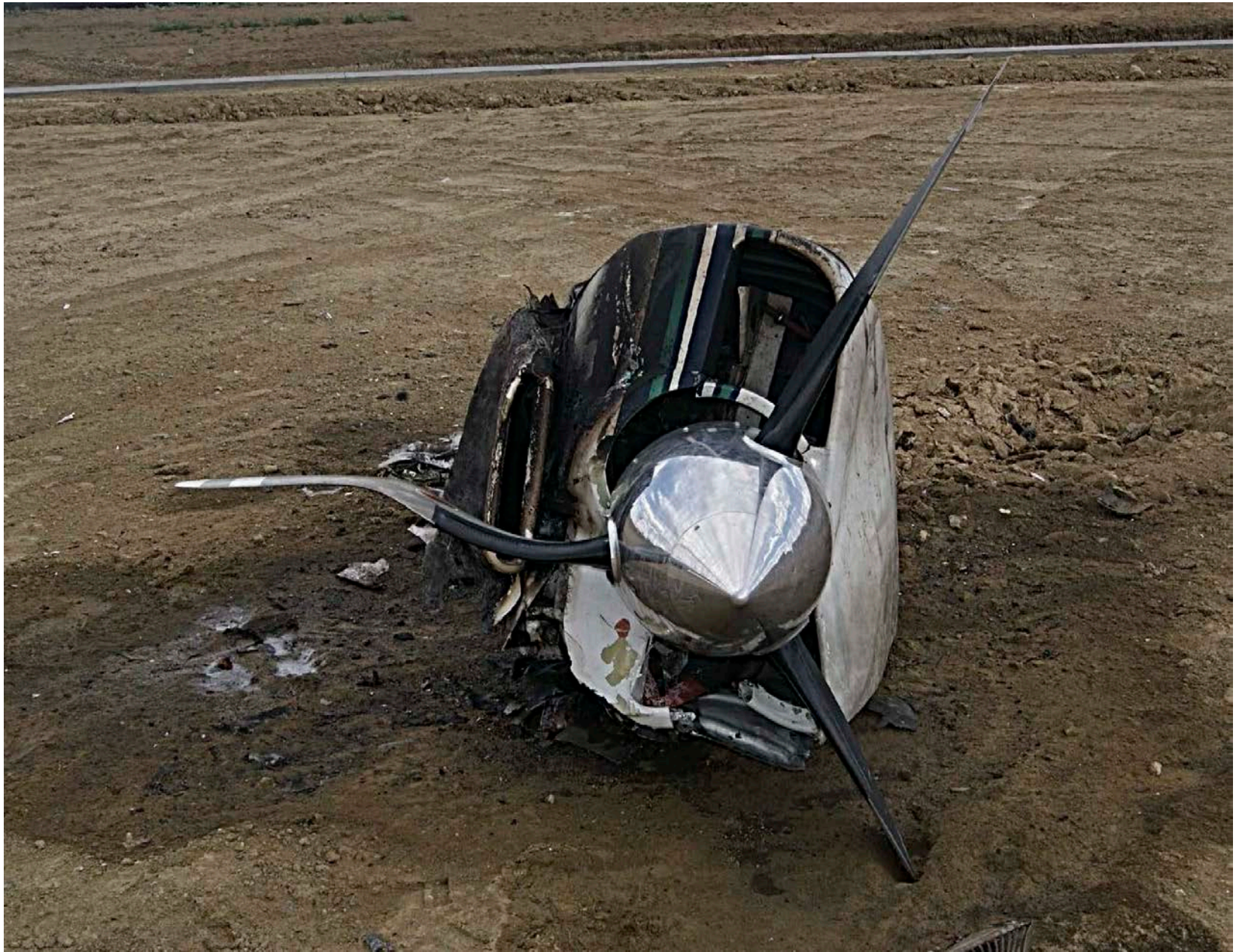
Photo 6 – The right engine. Note propeller is feathered.
