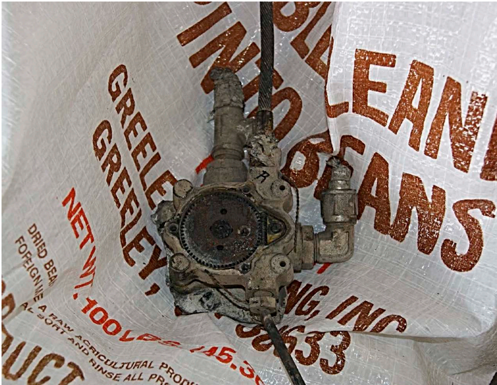
Photo 12 – Right engine fuel selector positioned on the right main tank.
