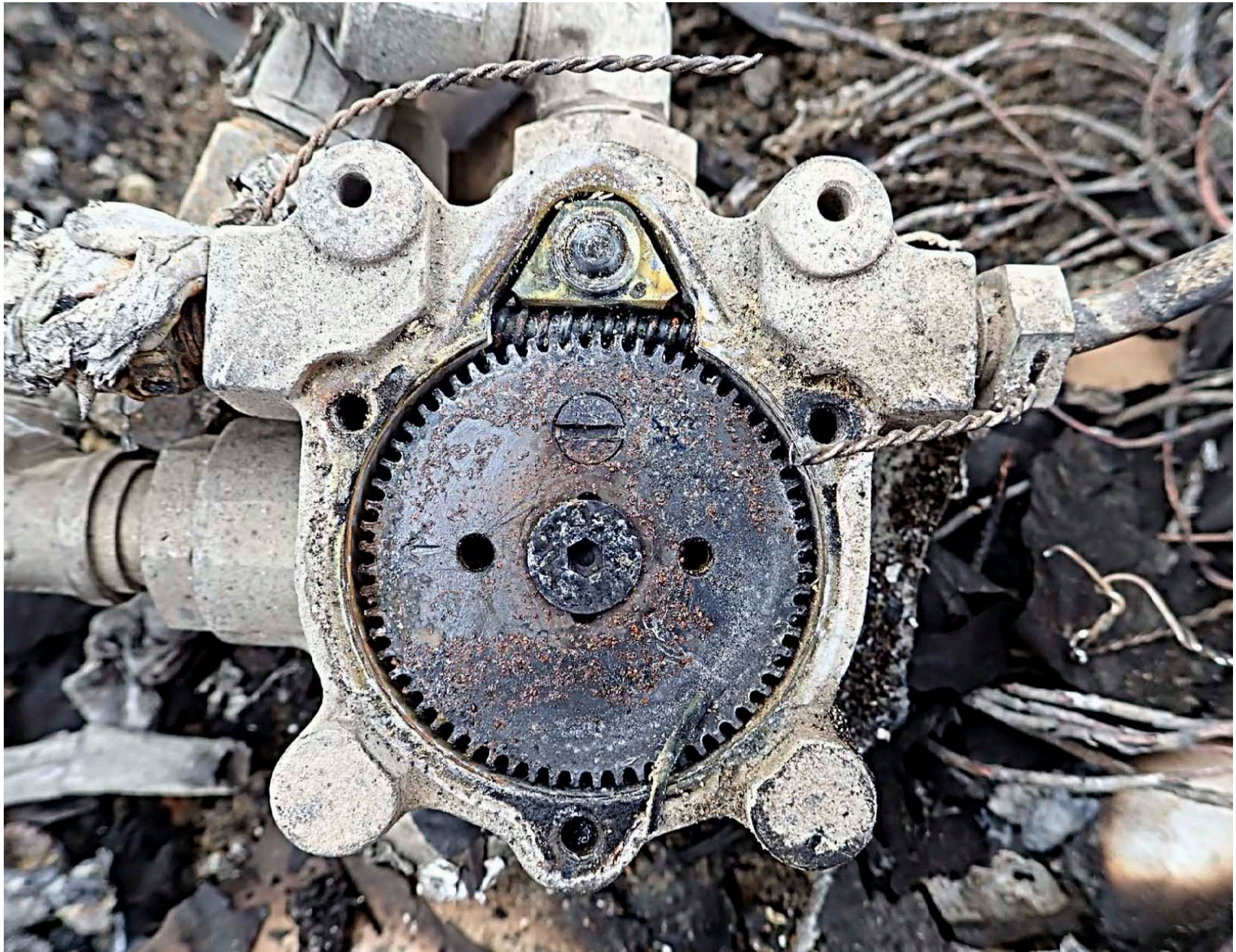
Photo 13 - Left engine fuel selector positioned on the left main tank.
