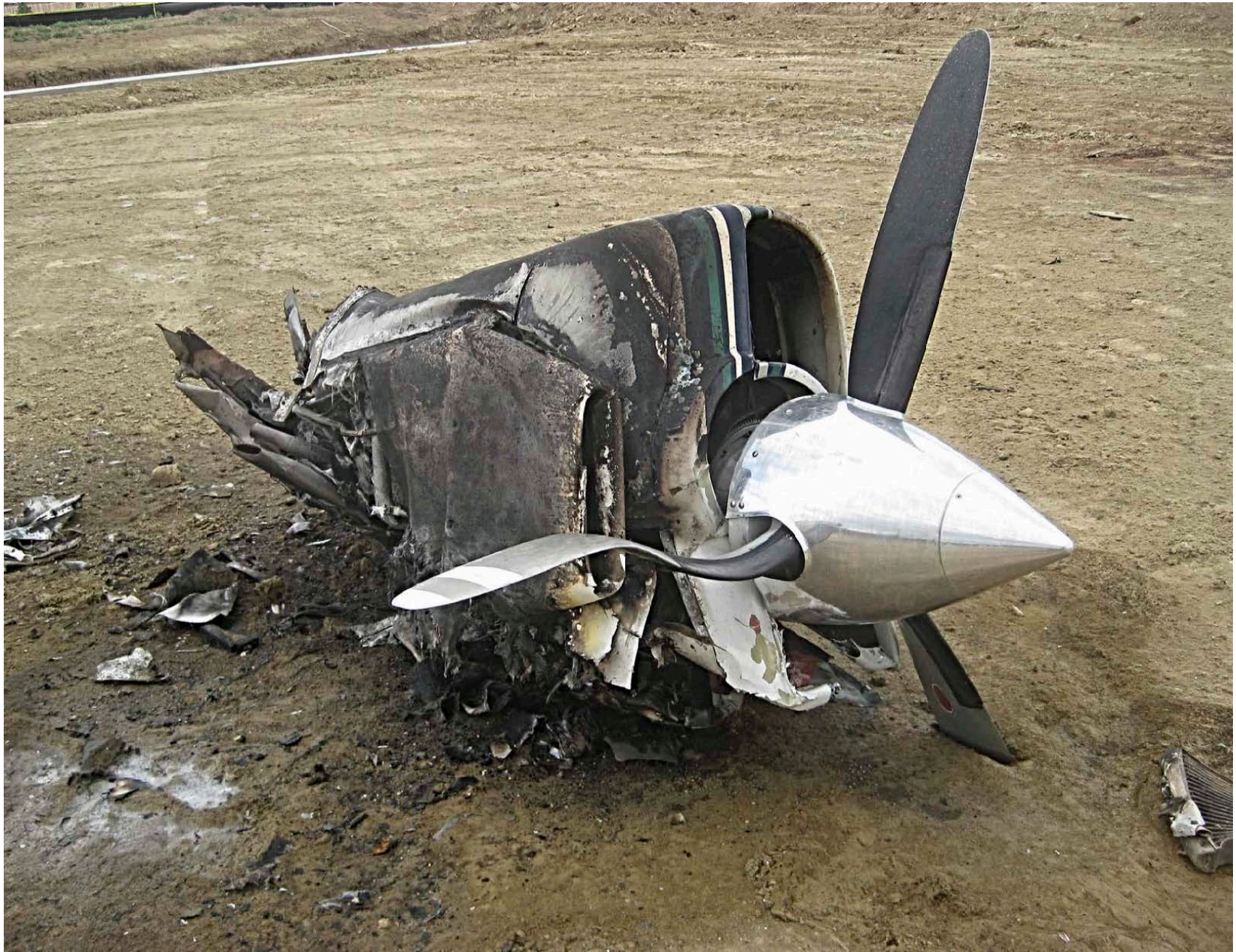
Photo 7 – Thermal damage to underside of right engine nacelle.
