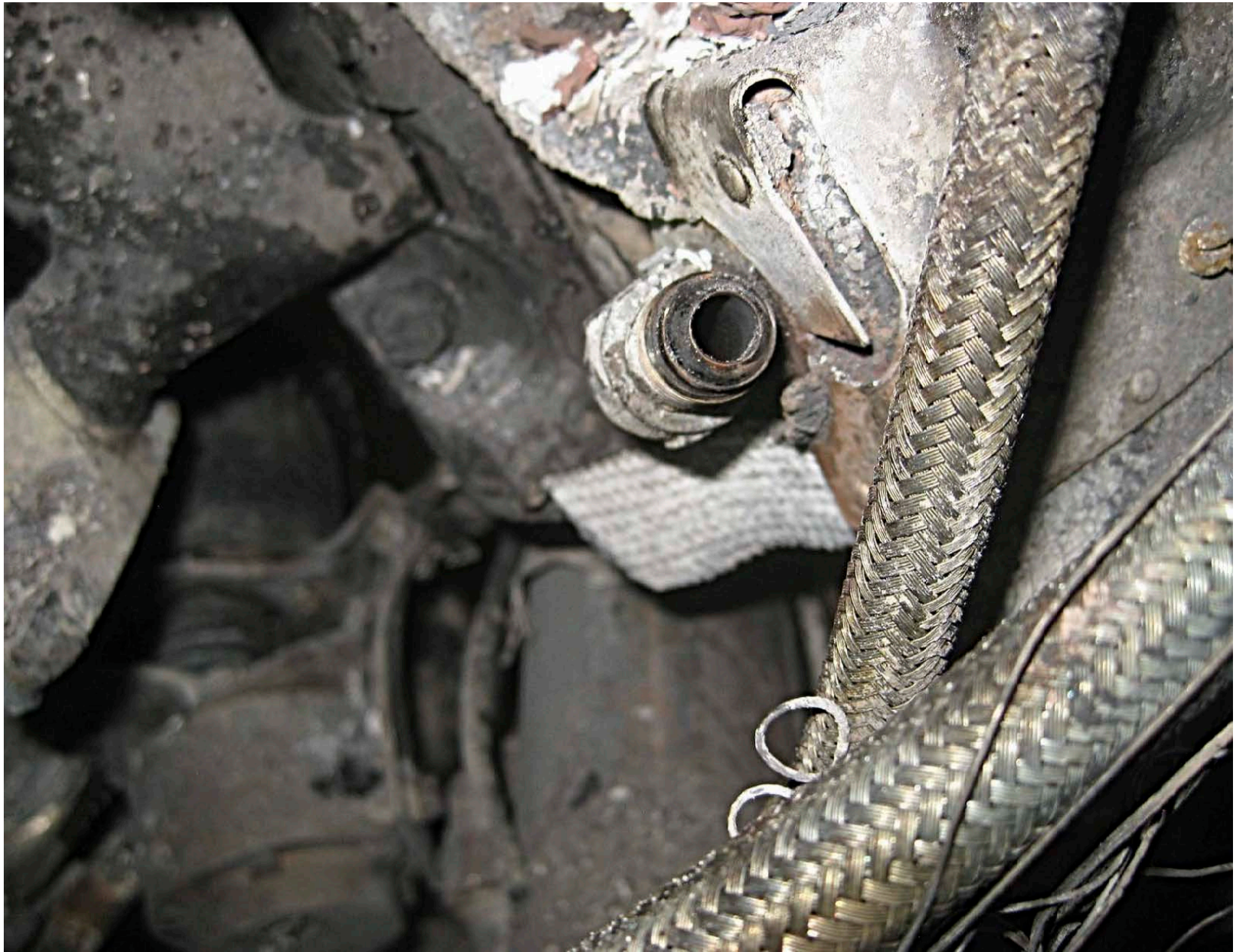
Photo 15 – Fuel pump discharge after line removal.
