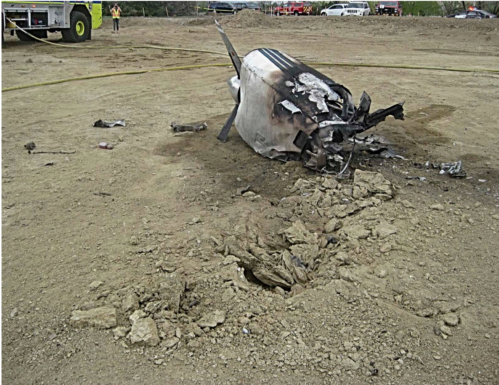
Photo 5 – The right engine and impact marks.
