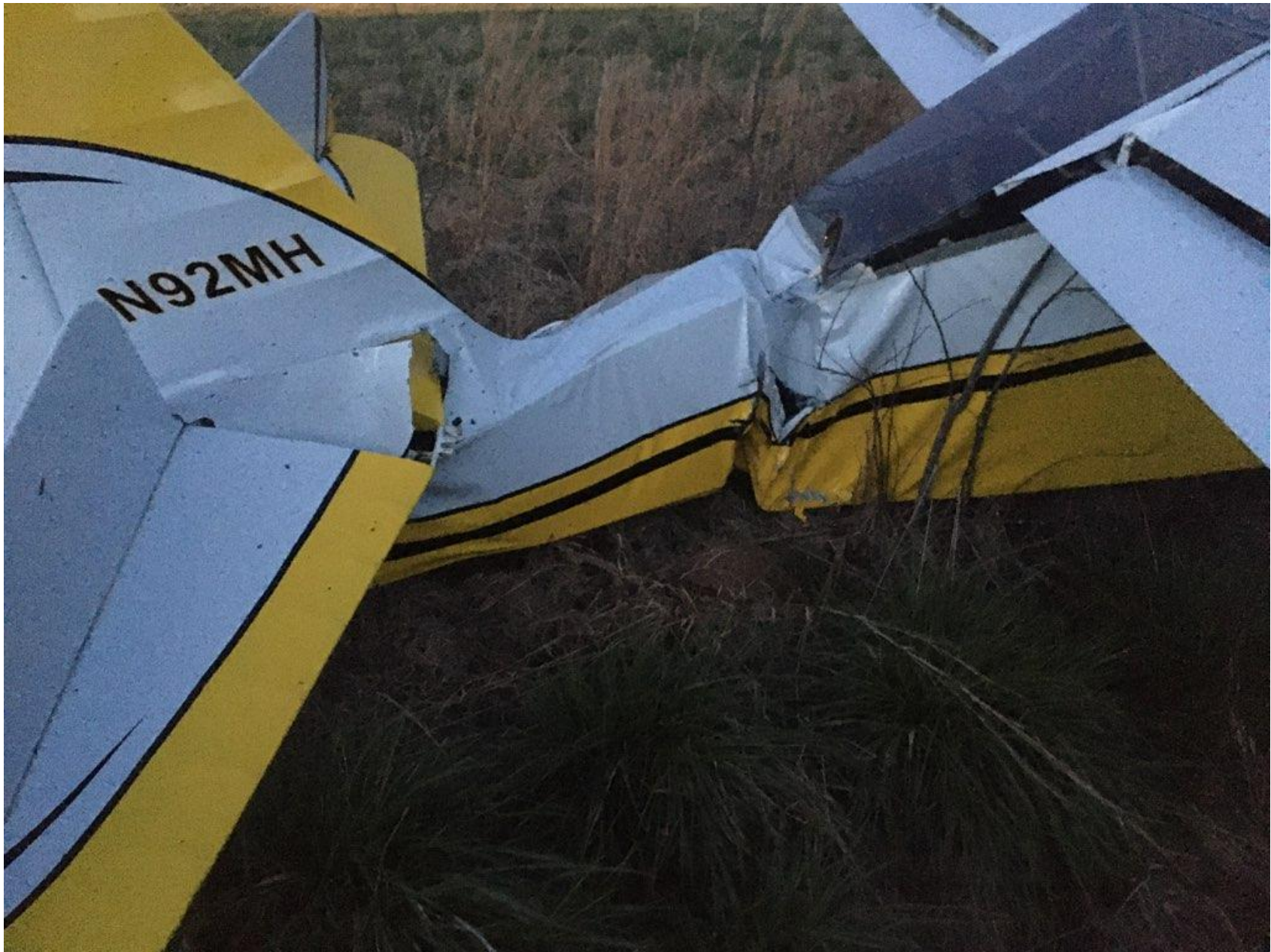
Photo 3 – Right side of N92MH and the buckled fuselage (FAA photo)
