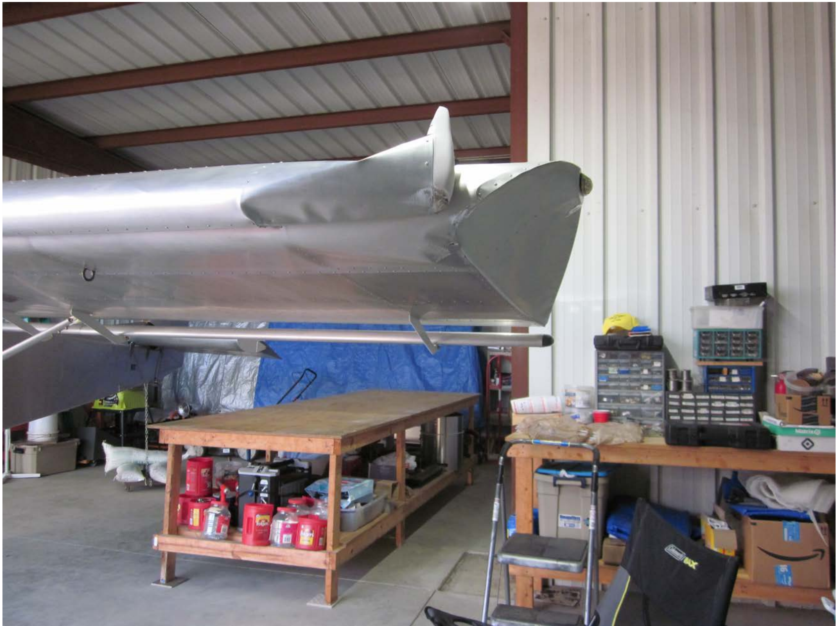
Photo 1 – Left wing tip damage (FAA photo)
